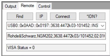
Figure 4-5 Remote configuration tab of a power supply
