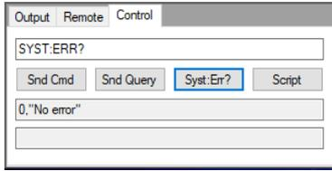
Figure 4-7 Remote control tab of a power supply
