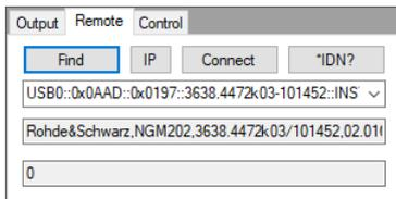
Figure 3-4 Remote configuration tab with R&S®NGM202 connected
