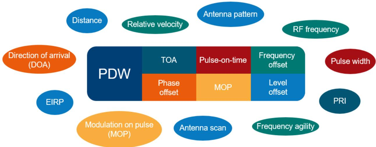
Figure 19: Overview of selected scenario, emitter and receiver parameters and their PDW parameter counterpart
