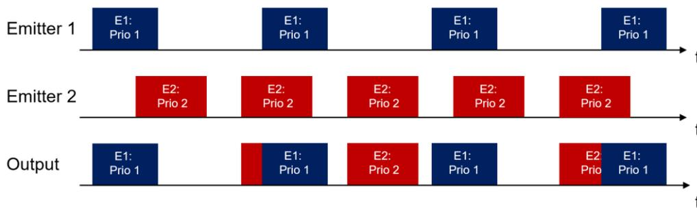
Figure 28: Priority based pulse dropping
