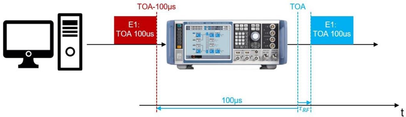
Figure 13: Timing diagram for PDW processing in the SMW200A
