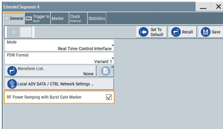
Figure 40: Configuration of the Burst Gate Marker in the Extended Sequencer configuration dialog
