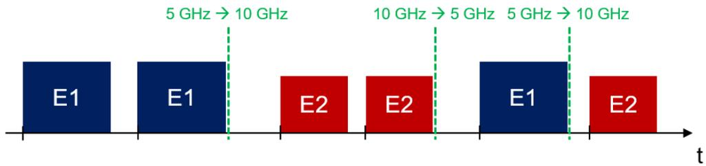
Figure 37: Simulation of two emitters at 5 GHz and 10 GHz
