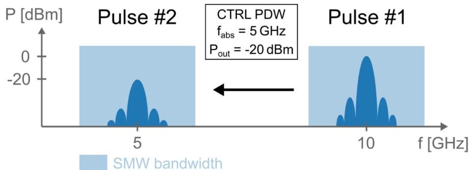
Figure 36: Switching RF level and RF frequency with TCDW
