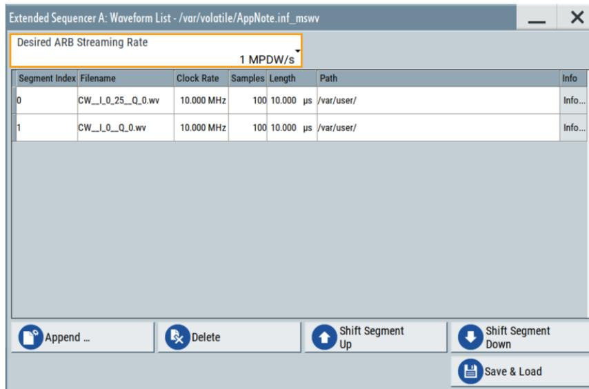
Figure 12: Waveform list configuration dialog in the SMW200A
