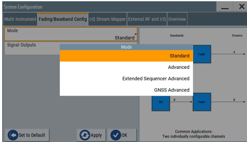
Figure 9. System configuration dialog in the SMW200A
