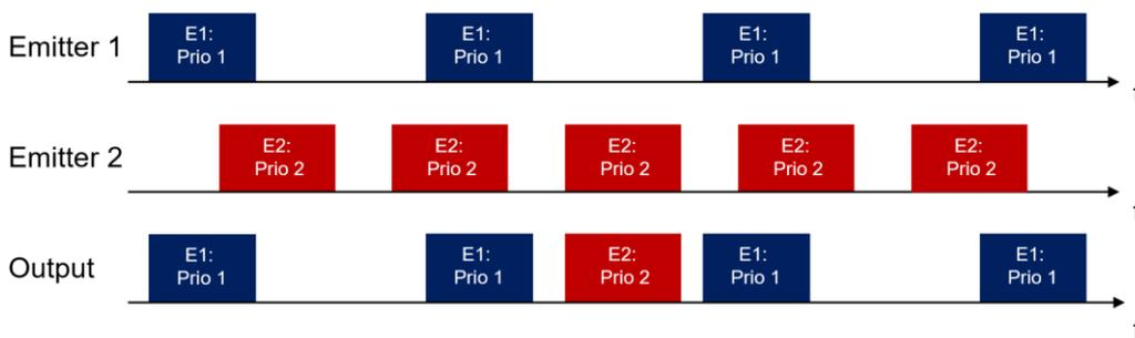
Figure 29: Priority based pulse dropping without interrupted PDWs
