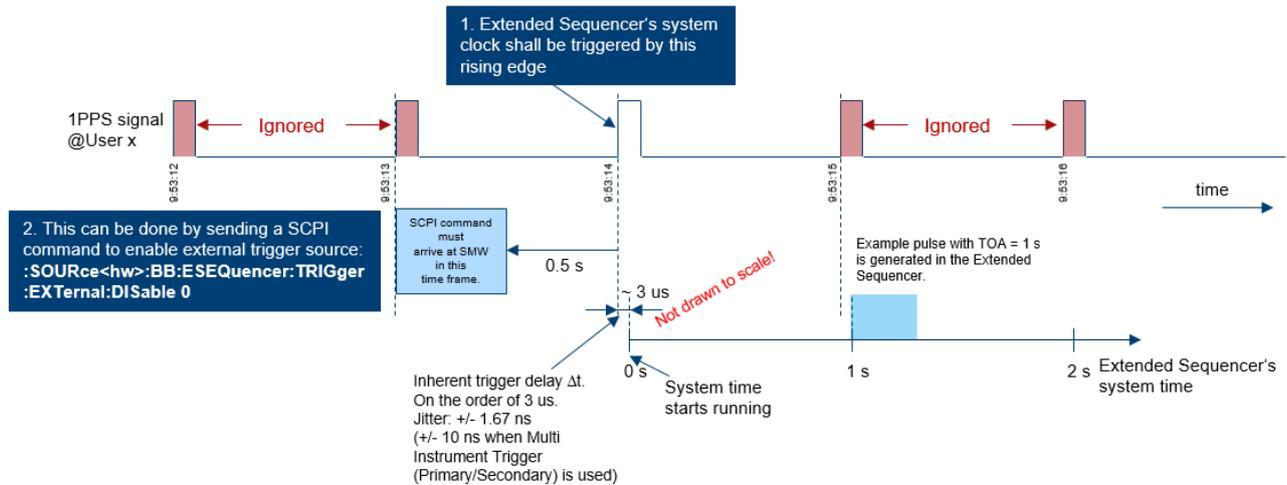
Figure 16: Timing diagram for triggering with a 1PPS signal
