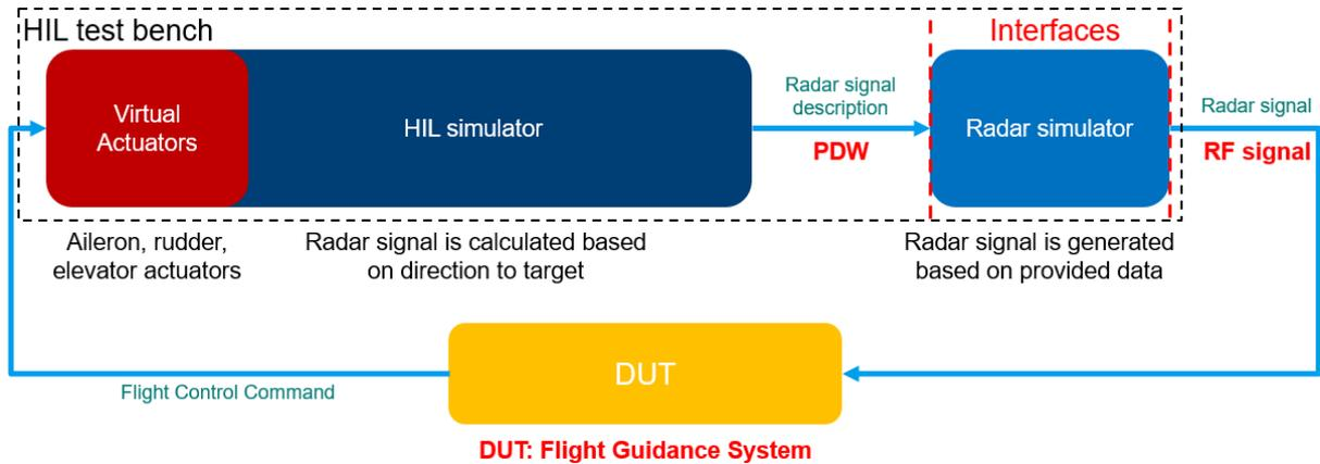
Figure 17: HIL test bench example for testing a flight guidance system
