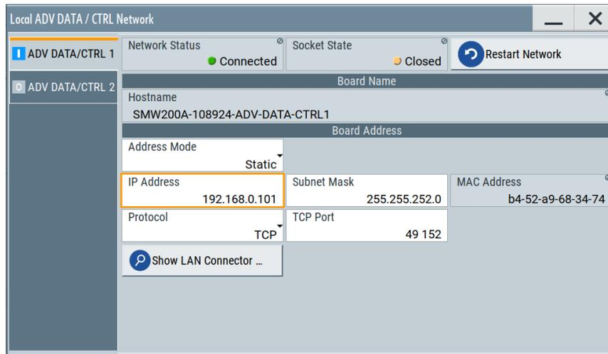
Figure 11: PDW interface configuration dialog in the SMW200A
