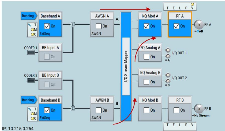
Figure 32: Block diagram showing the signal routing in the SMW200A
