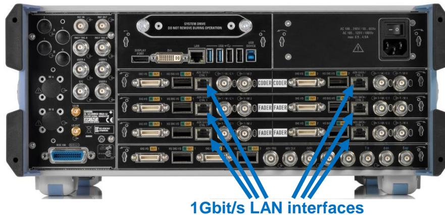
Figure 7: 1Gbit/s LAN interfaces on the SMW200A
