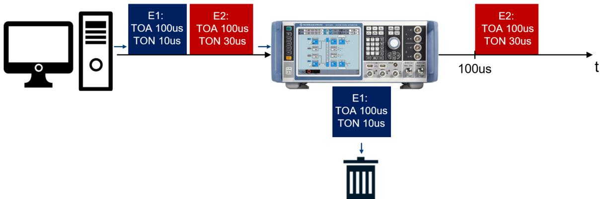
Figure 26: Pulse dropping: PDWs with same TOA parameter
