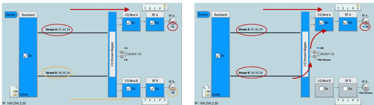
Figure 8: Possible routings of six independent PDW streams
