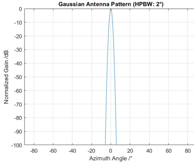
Figure 22: Normalized gain vs. azimuth angle of gaussian antenna
