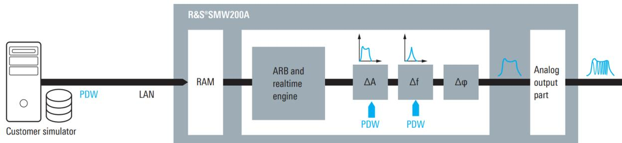
Figure 6: Concept of PDW streaming with the SMW200A
