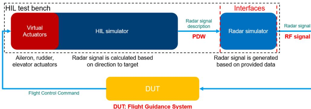
Figure 2: HIL test bench example for testing a flight guidance system
