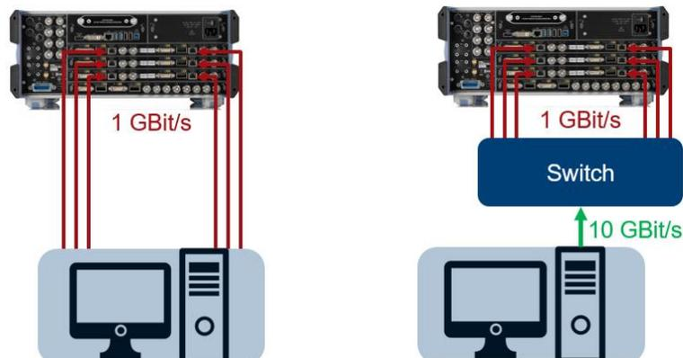
Figure 42: Possible network topologies for advanced PDW streaming
