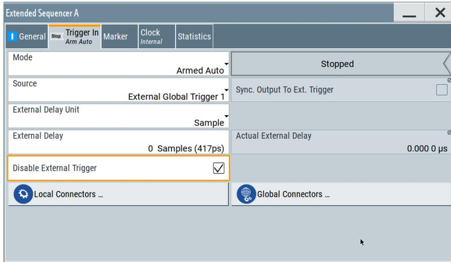
Figure 15: Trigger configuration dialog in the SMW200A
