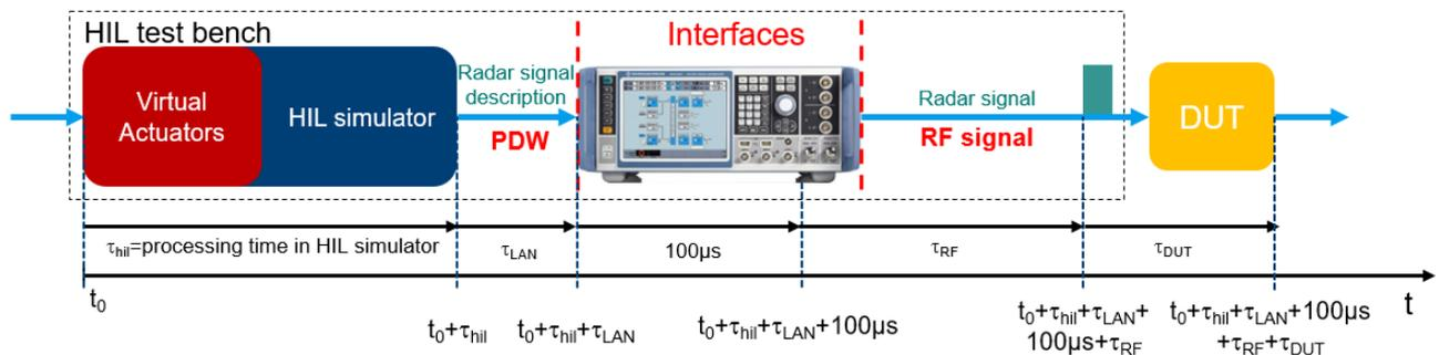
Figure 18: Contributions to loop latency in a HIL setup
