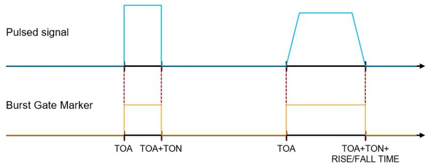
Figure 41: Illustration of Burst Gate Marker signal for pulsed signals
