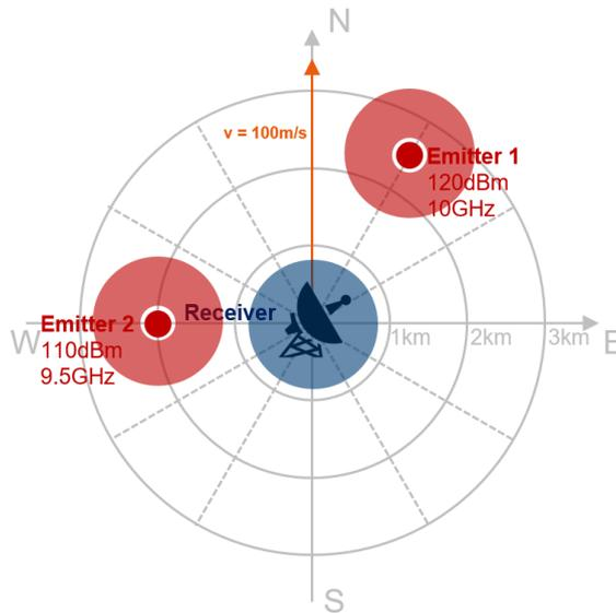
Figure 25: Scenario with two static threats and static receiver
