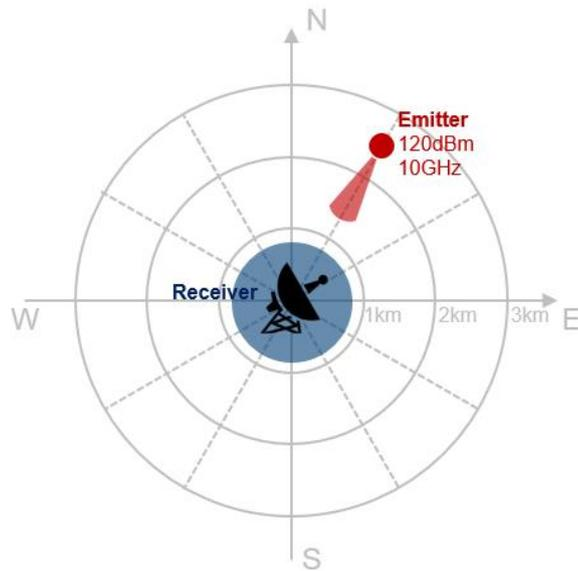
Figure 20: Scenario with static threat and static receiver
