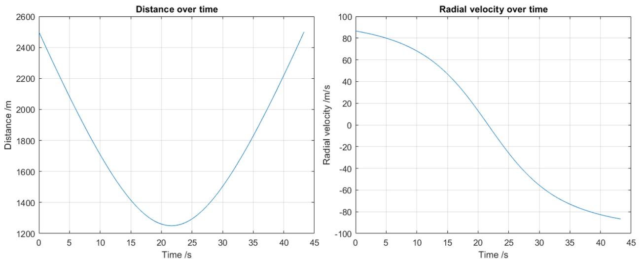
Figure 24: Relative distance and radial velocity between moving receiver and static emitter over time
