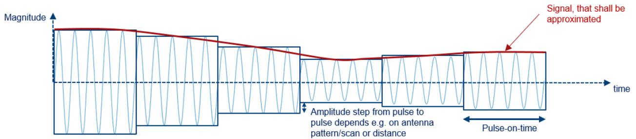
Figure 39: Concatenated PDWs to simulated CW interferer with changing signal amplitude
