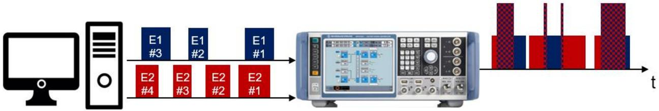
Figure 30: Pulse-on-pulse simulation on one RF output with two parallel PDW streams
