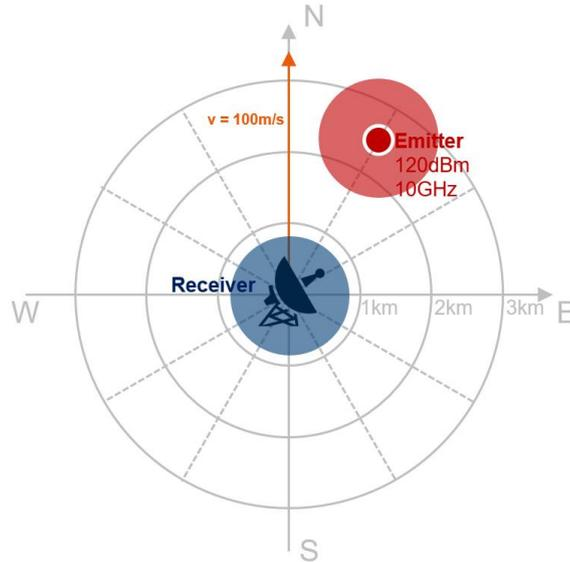
Figure 23: Scenario with static threat and moving receiver
