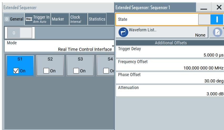
Figure 44: Extended Sequencer Advanced configuration dialog in the SMW200A
