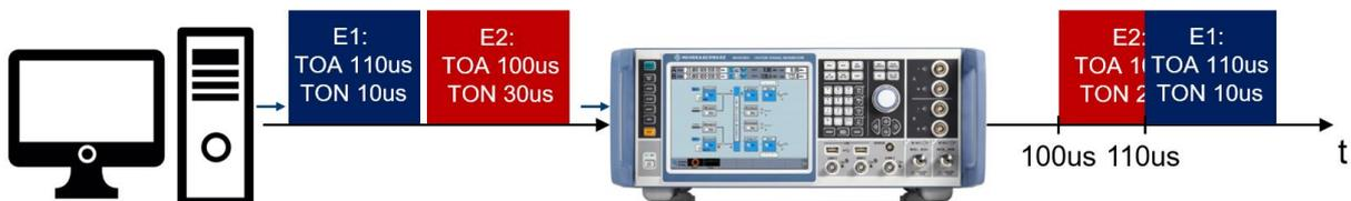
Figure 27: Pulse dropping: PDW with TOA parameter before preceding PDW is finished
