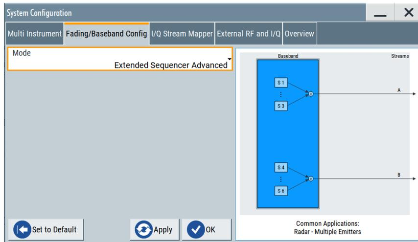
Figure 43: System configuration dialog in the SMW200A
