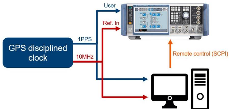
Figure 14: GPS based synchronization of HIL simulator and SMW200A
