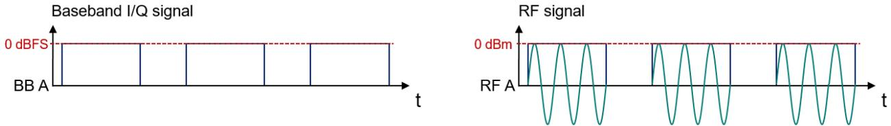
Figure 33: SMW level setting with single I/Q signal from baseband A (BB A) assigned to RF path A
