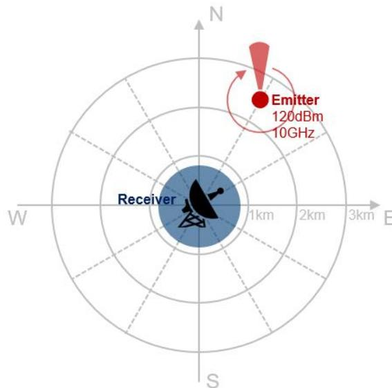
Figure 21: Scenario with static threat with circular antenna scan and static receiver
