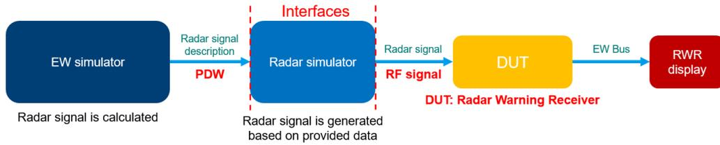
Figure 4: Open-loop testing of a radar warning receiver
