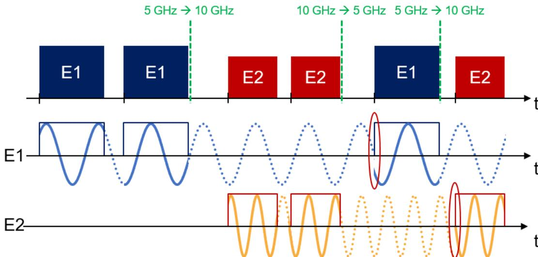
Figure 38: Phase of two emitters at 5 GHz and 10 GHz
