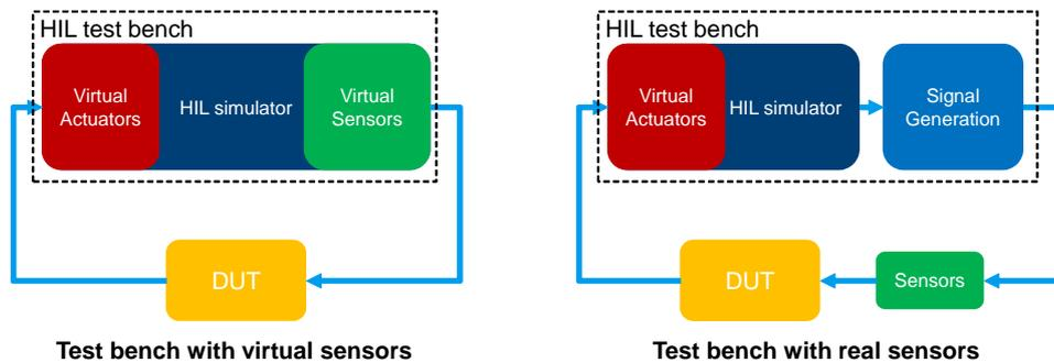
Figure 1: Block diagrams for HIL test benches with virtual and real sensors
