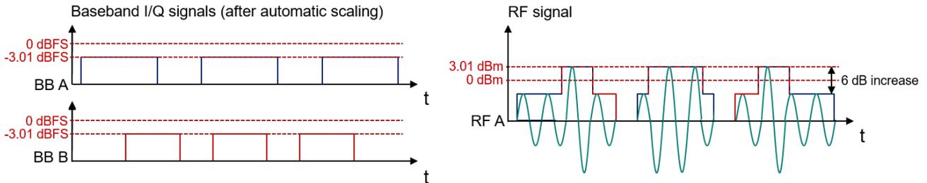
Figure 34: SMW level setting with two I/Q signals from baseband A (BB A) and B (BB B) assigned to RF path A
