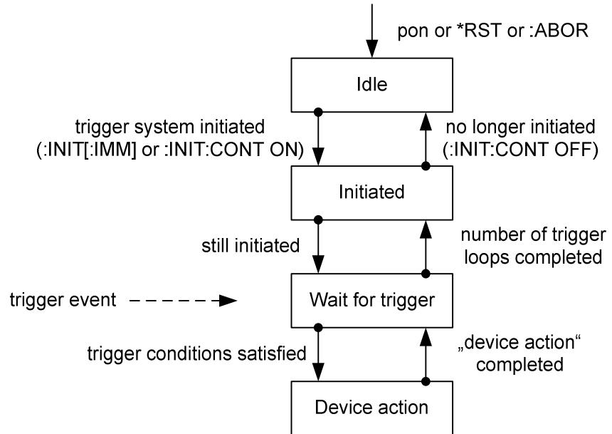
Other emulated instruments and also the SMA100B implement the trigger control system shown in the following figure:
