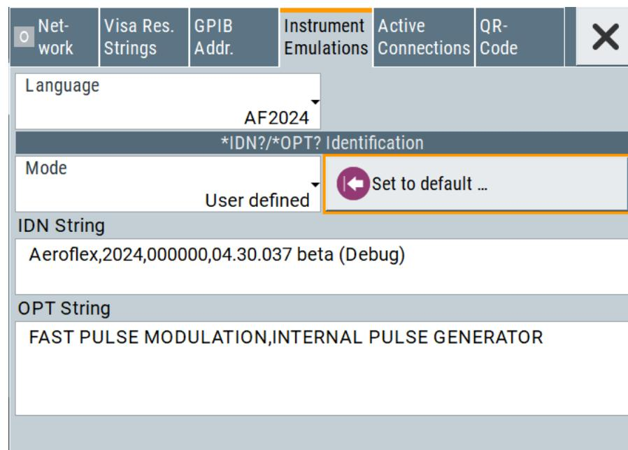
Then select the IDN String text box and edit the response text to \*IDN? queries. When finished, confirm the text:
