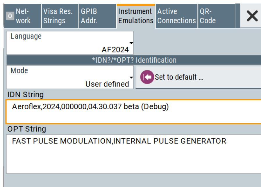
Finally select the OPT String text box and edit the response text to \*OPT? queries. When finished, confirm the text:
