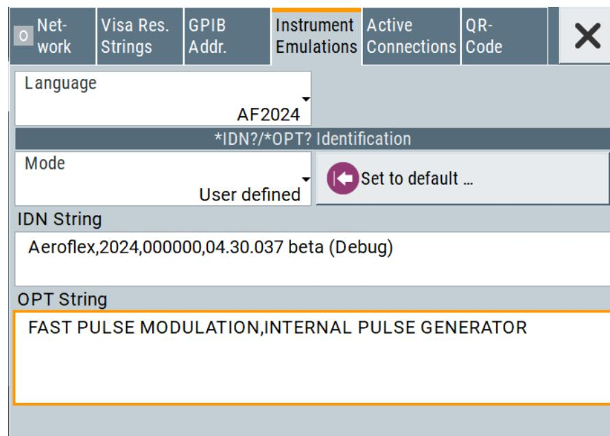
Exit the Instrument Emulations dialog by pressing the ESC key and verify the selected remote emulation on the SMA100B front panel:
