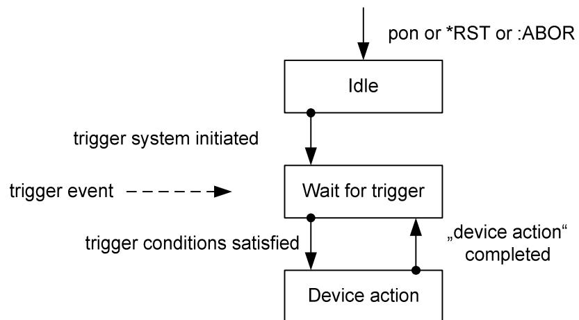
The main difference between the emulated instrument's and the SMA100B's trigger control system is that there is no “Initiated” state in the SMA100B. The SMA100B implementation assumes that the trigger system is initiated automatically in the “Idle” state. As a result, any sweep operation in the SMA100B, once activated, can only be controlled by internal or external trigger events.
