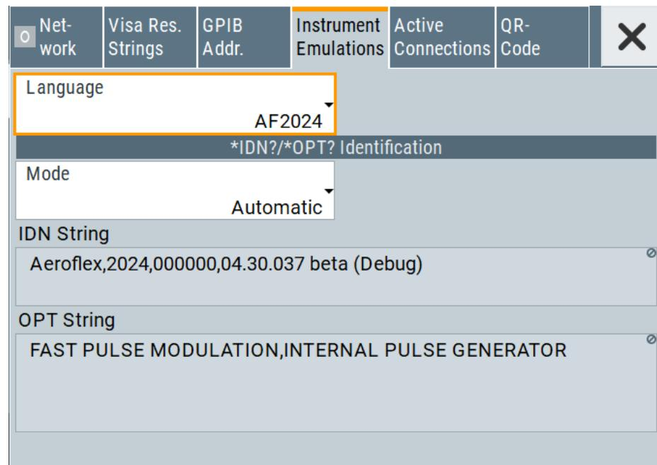
Select the Mode and open the drop-down list. Pick either "Automatic" or "User defined" from the list and confirm the selection.
