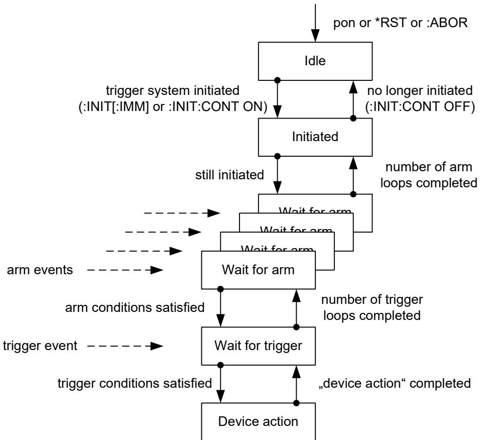
Some of the emulated instruments implement a simplified trigger control system:
