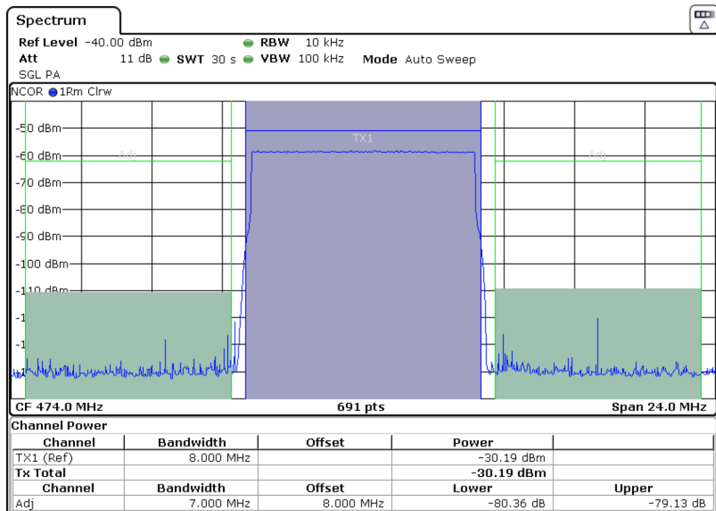
Fig. A-3: ACLR measurement for adjacent channel separation test 4
