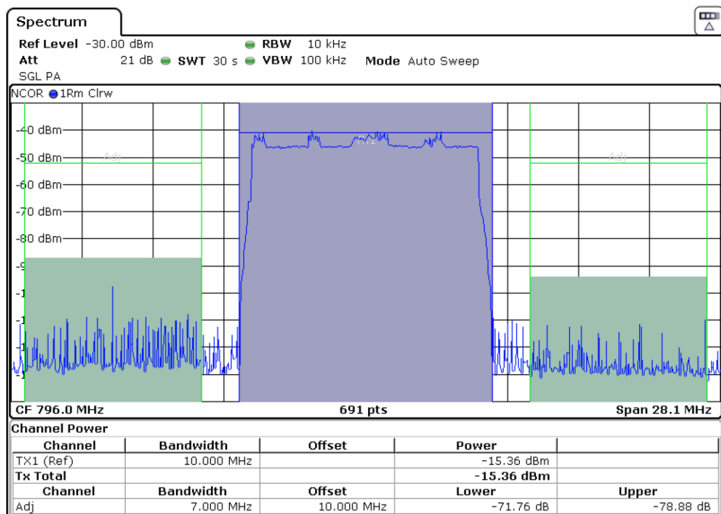
Fig. A-1: ACLR measurement for adjacent channel separation test 1
