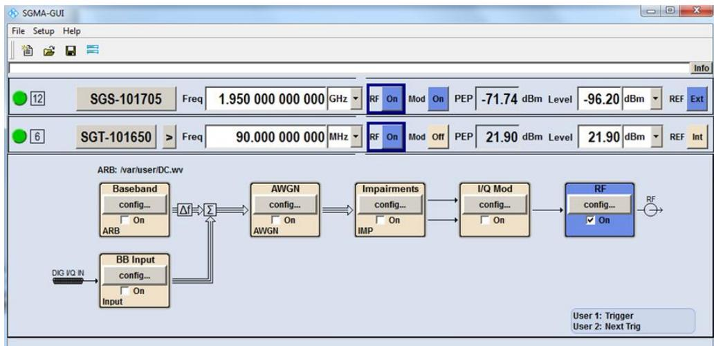
The PC software can control multiple instruments at once and provides full instrument control (e.g. including firmware update).
