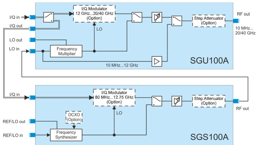
The I/Q signals from an external ARB generator are fed into the SGU. For frequencies below 12 GHz the I/Q signal is routed to the SGS.
