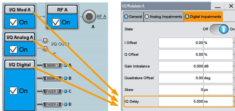
The "I/Q Delay" parameter delays the baseband signal with picosecond resolution. By adjusting this parameter the RF output signals can be perfectly aligned in time, if required for the application.
