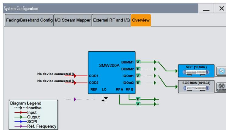
The diagram shows the input and output connectors of the SMW. For each output connector it shows
