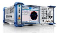
The SMBV is a cost-efficient general-purpose vector signal generator with outstanding RF performance capable of generating signals for all main communications and radio standards. Equipped with one or more GNSS options, the SMBV is also a full-fledged satellite signal simulator for reliable and flexible GNSS receiver testing. Please see reference [2] for more product details and feature set.
