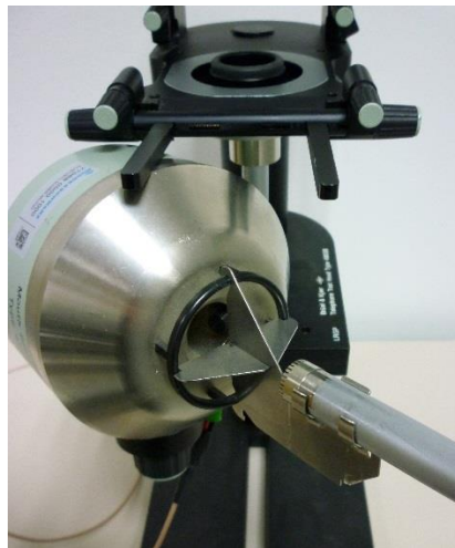
Fig. 2-4: Position of a free-field microphone for the calibration of the P.51 artificial mouth
