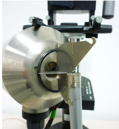
Fig. 2-3: Position of a diffuse-field or pressure-field measurement microphone for the calibration of the P.51 artificial mouth
