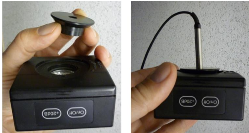
Fig. 2-2: Insertion of a 1/4" measurement microphone into the calibrator with adapter
