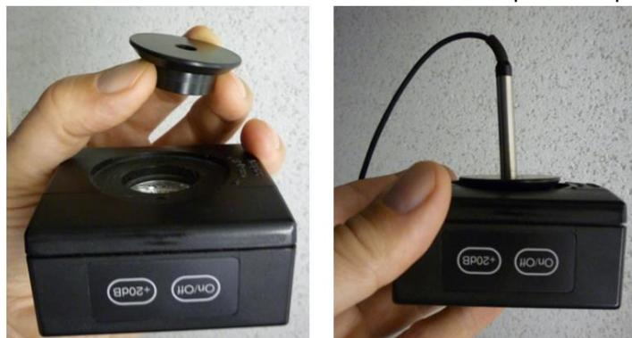
Fig. 2-7: Insertion of a ¼” measurement microphone into the calibrator with adapter
