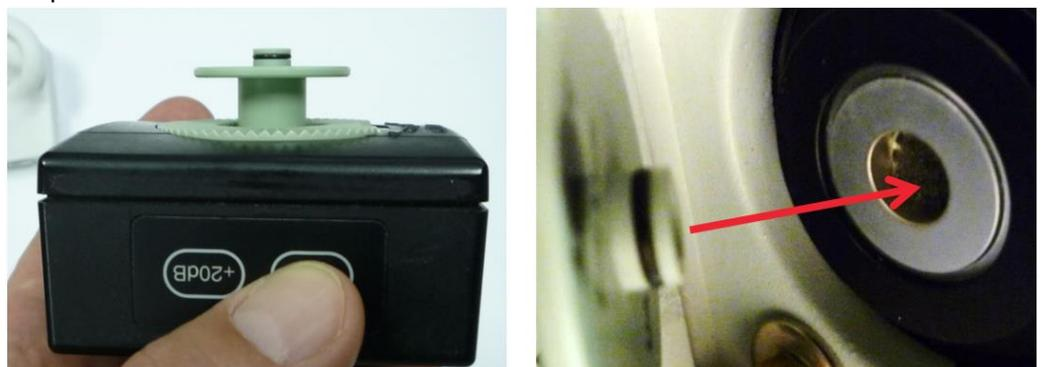
Fig. 2-10: Insertion of the calibrator with adapter into the ear simulator
