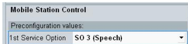
Figure 4 Setting the service option in the main page of CDMA2000 signalling
