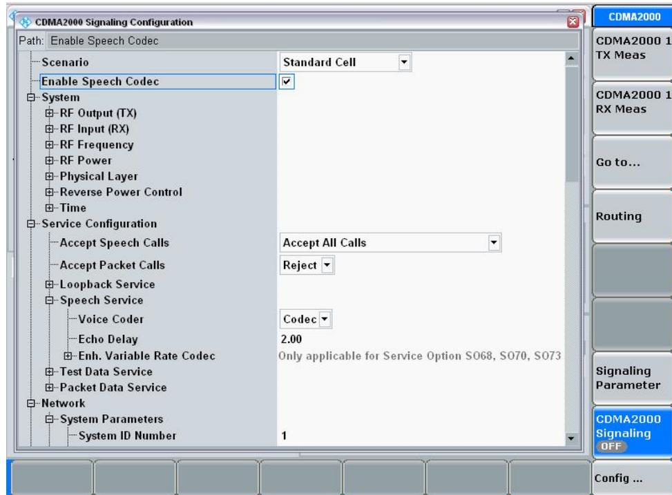
Figure 5 Setting the parameters for narrowband speech (SO3) on the CMW500
