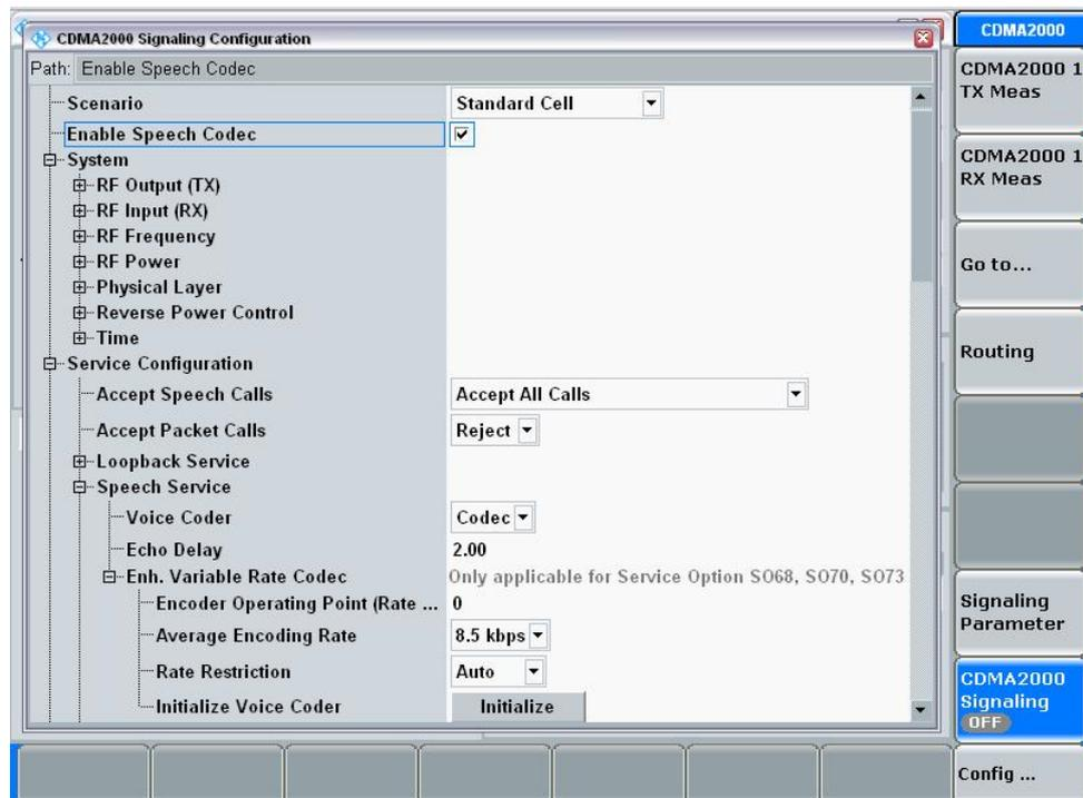
Figure 6 Setting the parameters for wideband speech (SO73 COP 0) on the CMW500
