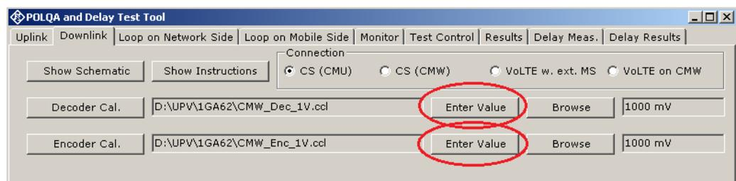
Figure 8 Buttons for direct entry of decoder and encoder calibration values
