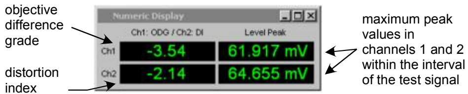
Figure 21: Numeric display of PEAQ results
