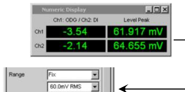
Figure 28: Correct setting of measurement range
