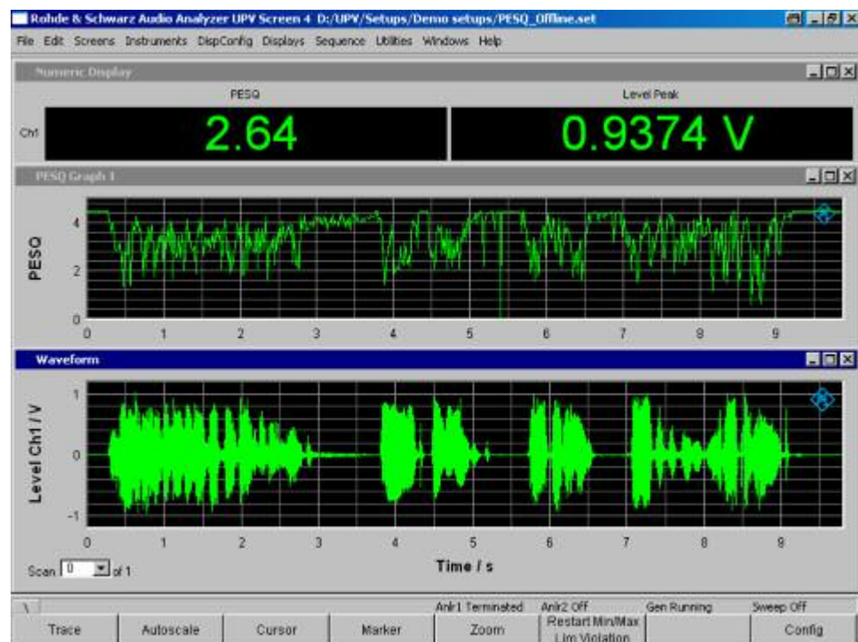
Figure 9: Graphical displays show PESQ values and/or the waveform versus time
