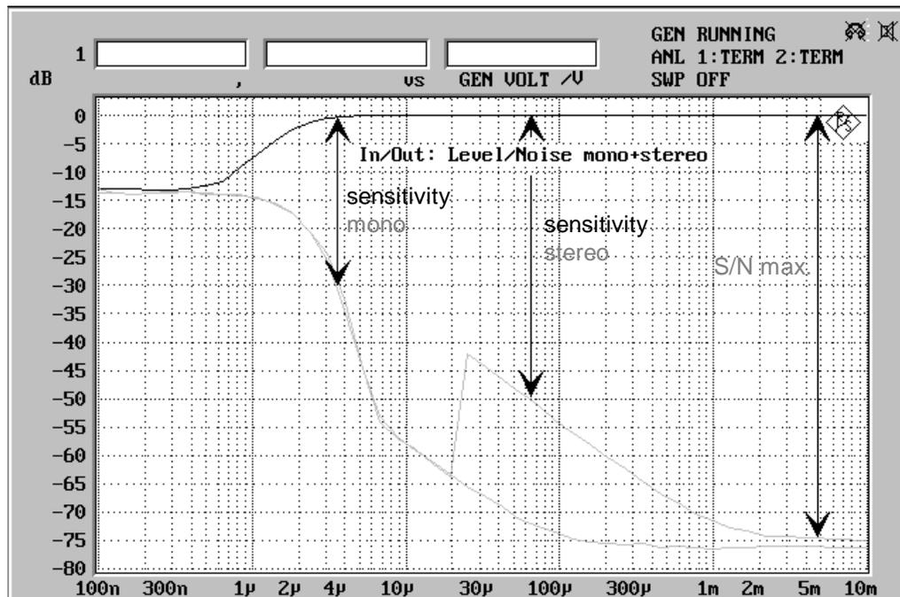
Fig. 8: Output/input signal characteristic of a tuner of the medium-price class
