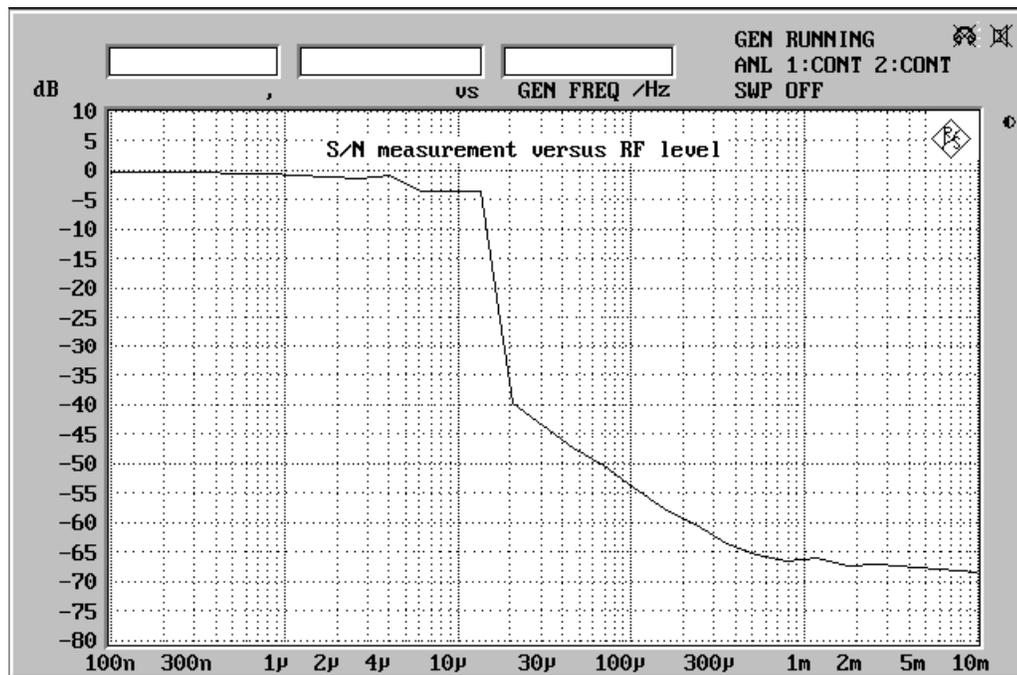
Fig. 7: S/N ratio as a function of modulation frequency
