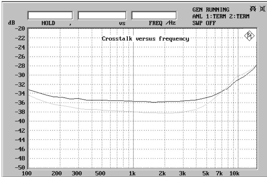
Fig. 5: Crosstalk attenuation as a function of modulation frequency
