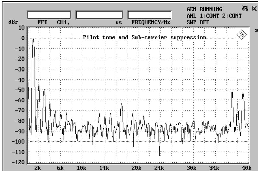
Fig. 9: Output spectrum of a tuner for 1-kHz modulation with pilot tone and subcarrier
