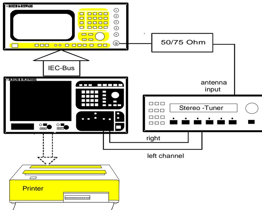
Fig. 1: Test setup for automatic tuner measurements
