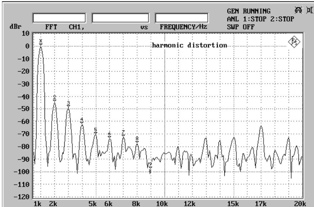
Fig. 3: Harmonic distortion of a 1-kHz signal
