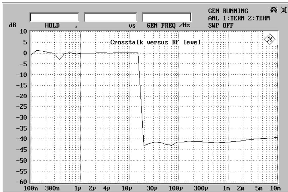
Fig. 6: Crosstalk attenuation as a function of RF level
