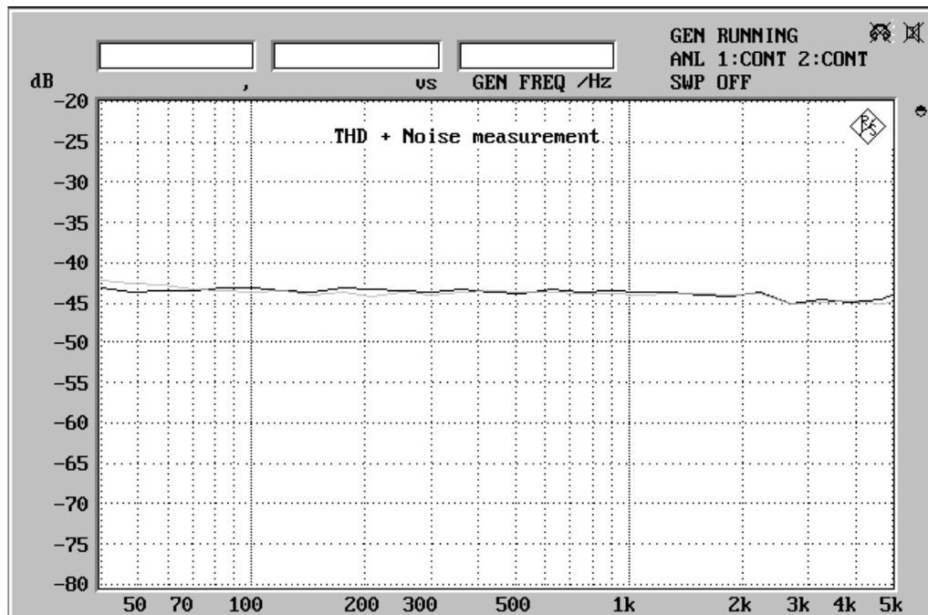
Fig. 2: THD+N measurement as a function of modulation frequency
