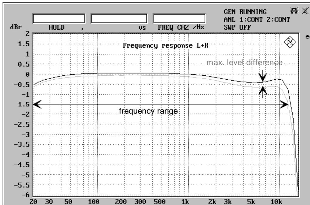
Fig. 4: Audio frequency response of a stereo receiver referred to the 1-kHz value of the right channel
