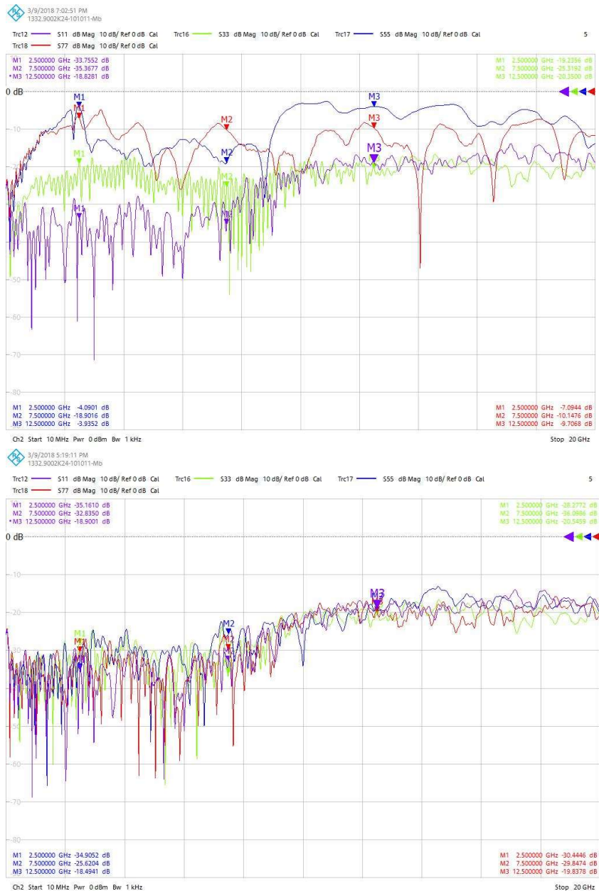
Figure 19: Single Ended Return Loss S11 of the Undesired Degraded Backplane vs. the Desired Clean Backplane
