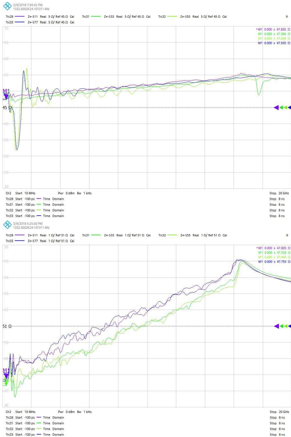
Figure 22: TDR Plots of Ports 1, 3, 5 and 7
