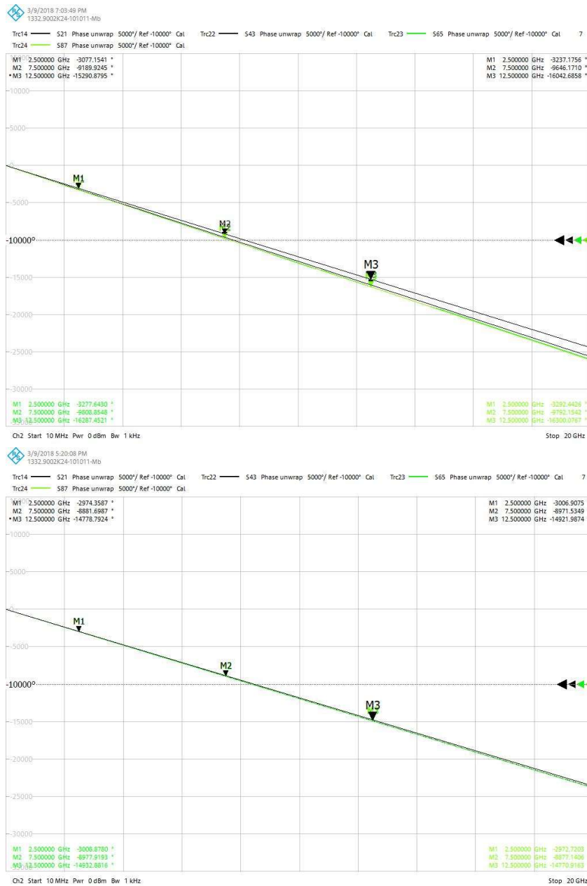
Figure 21: Single Ended Insertion Loss S_{21} Unwrapped Phase of the Undesired Degraded Backplane vs. the Desired Clean Backplane
