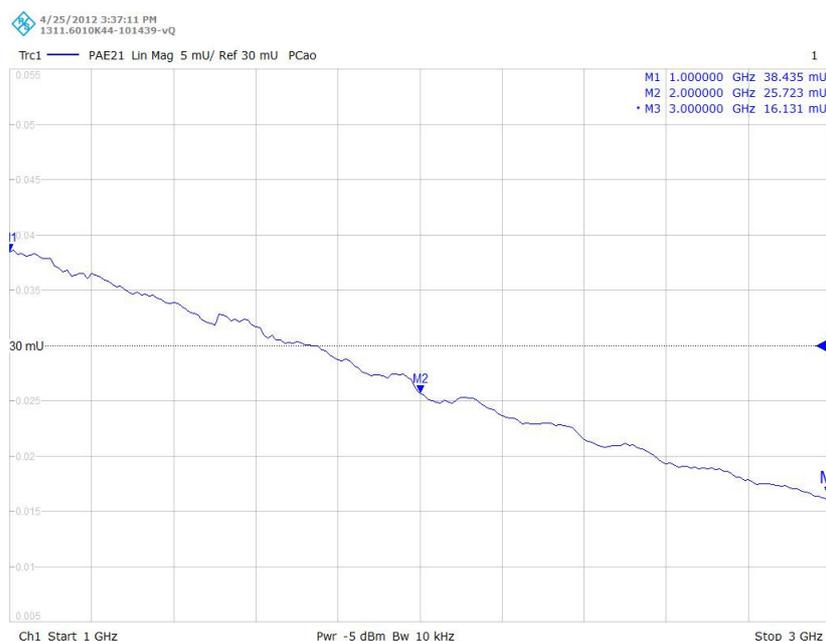
Figure 4: Measurement result of the PAE versus frequency based on DC function
