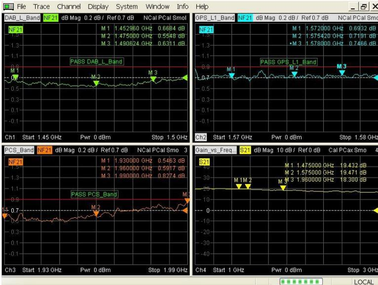
Noise figure measurement in the DAB-L band
