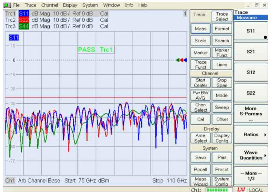
Fig. 4.10: Automatic limit check of return loss for all ports of the directional coupler
