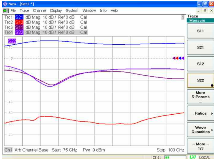
Fig. 4.17: Measurement results obtained for an IAF MDMAW01BM amplifier
