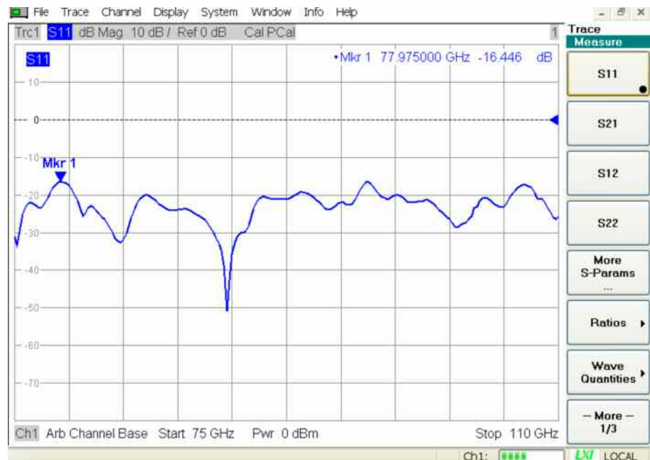
Fig. 4.12: Measuring return loss on the RF port of an R&S® FS-Z110 mixer
