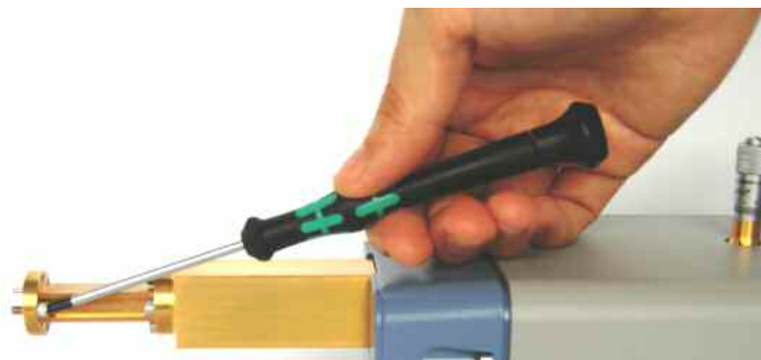
Fig. 4.5: Screwing a waveguide flange to its counterpart, e.g. a DUT
