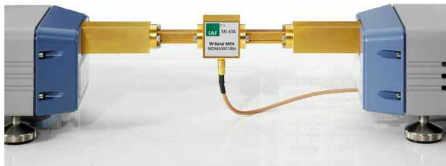
Fig. 4.16: Amplifier mounted between two R&S® ZVA-Z110 converters (DUT by courtesy of Fraunhofer Institute for Applied Solid-State Physics, Freiburg/Germany)
