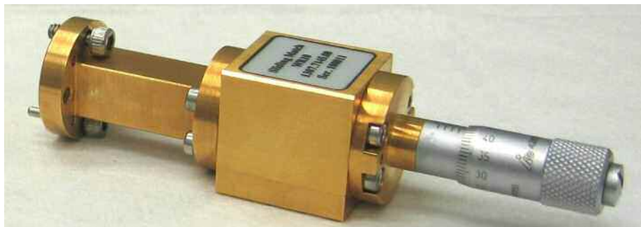
Fig. 4.11: Waveguide sliding match of the R&S® ZV-WR10 calibration kit set to 0.35 mm
