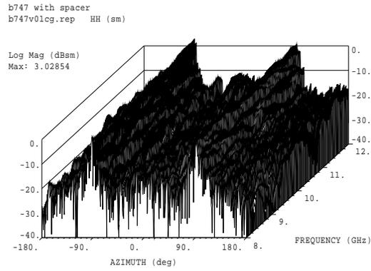
Figure 20: RCS response for  $\pm 180^\circ$  and 8-12 GHz.
