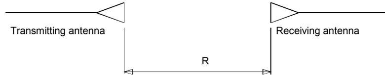
**Figure 1:** Orientation of transmitting and receiving antennas aligned for maximum directional radiation and reception.
