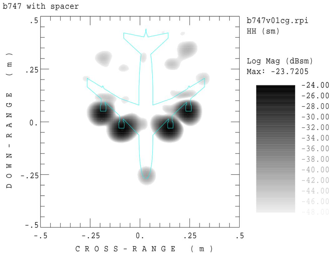
Figure 21: ISAR image of a B747 (1:100 scale).
