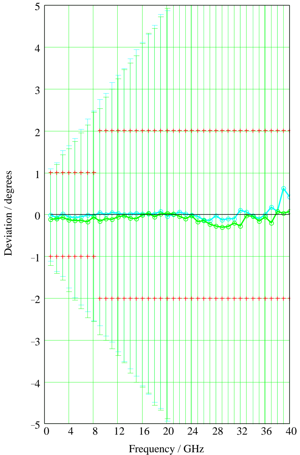
Fig. 4-2 Transmission phase deviations: 2.92 mm 50 \Omega airline verification standard at 0 dB
