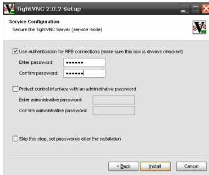
After installation of the TightVNC on the R&S<sup>®</sup> RTO a reboot of the instrument is required.
