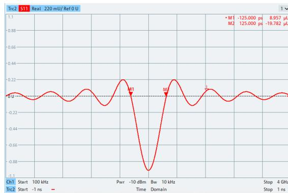
Fig. 22 Width of si pulse ( $\Delta F = 4$  GHz) halved in lowpass mode in comparison with Fig. 18. The pulse width  $\Delta T$  is now approx. 250 ps.
