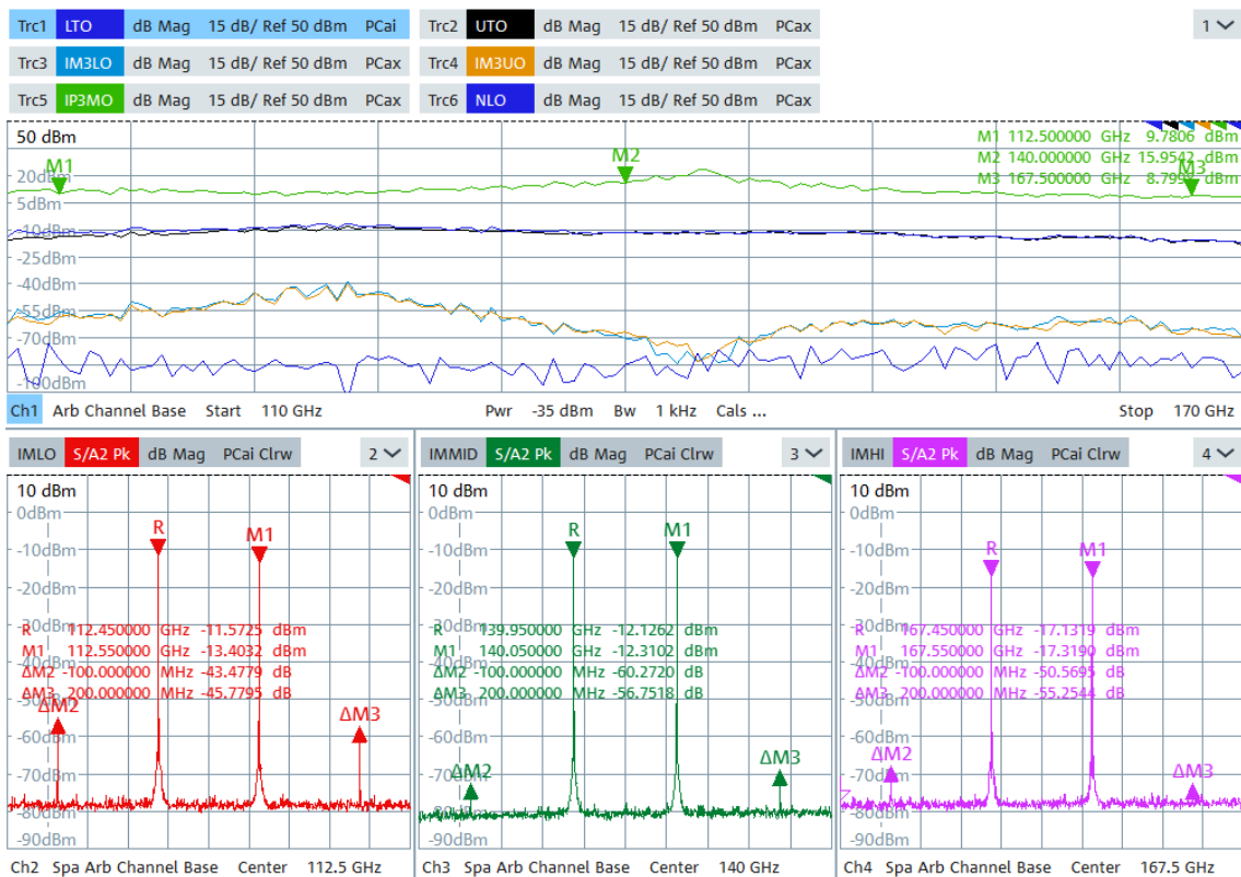
Fig. 31: Intermodulation measurement of a D-band LNA
