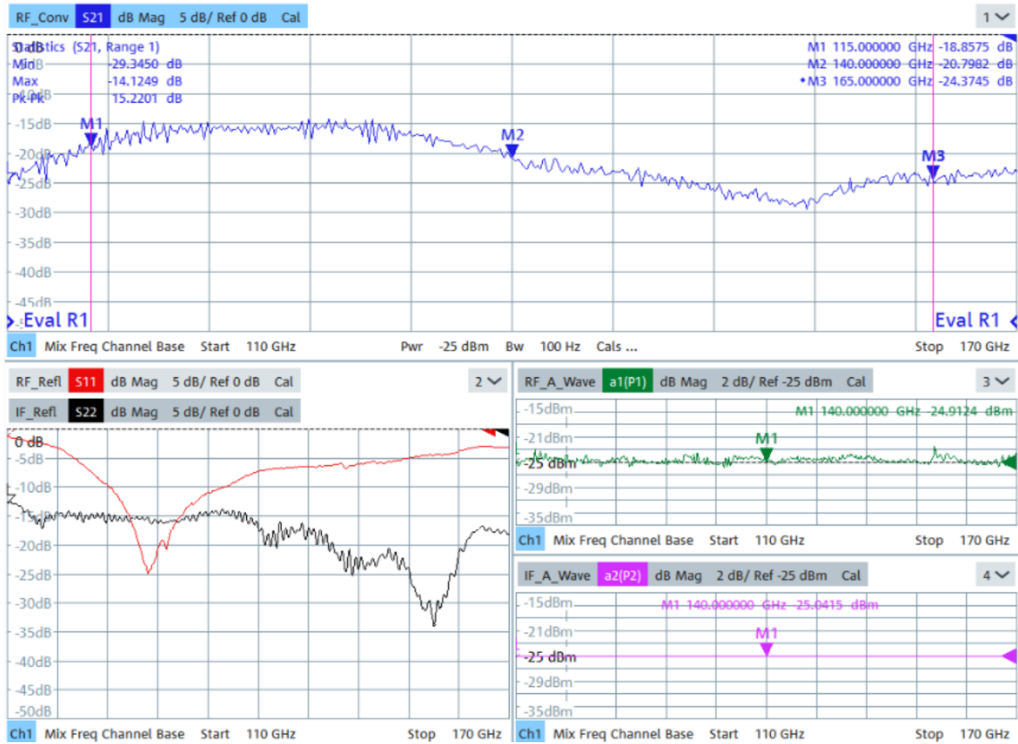
Fig. 24: Magnitudes of mixer S-parameters after scalar mixer calibration + incident waves of RF and IF port
