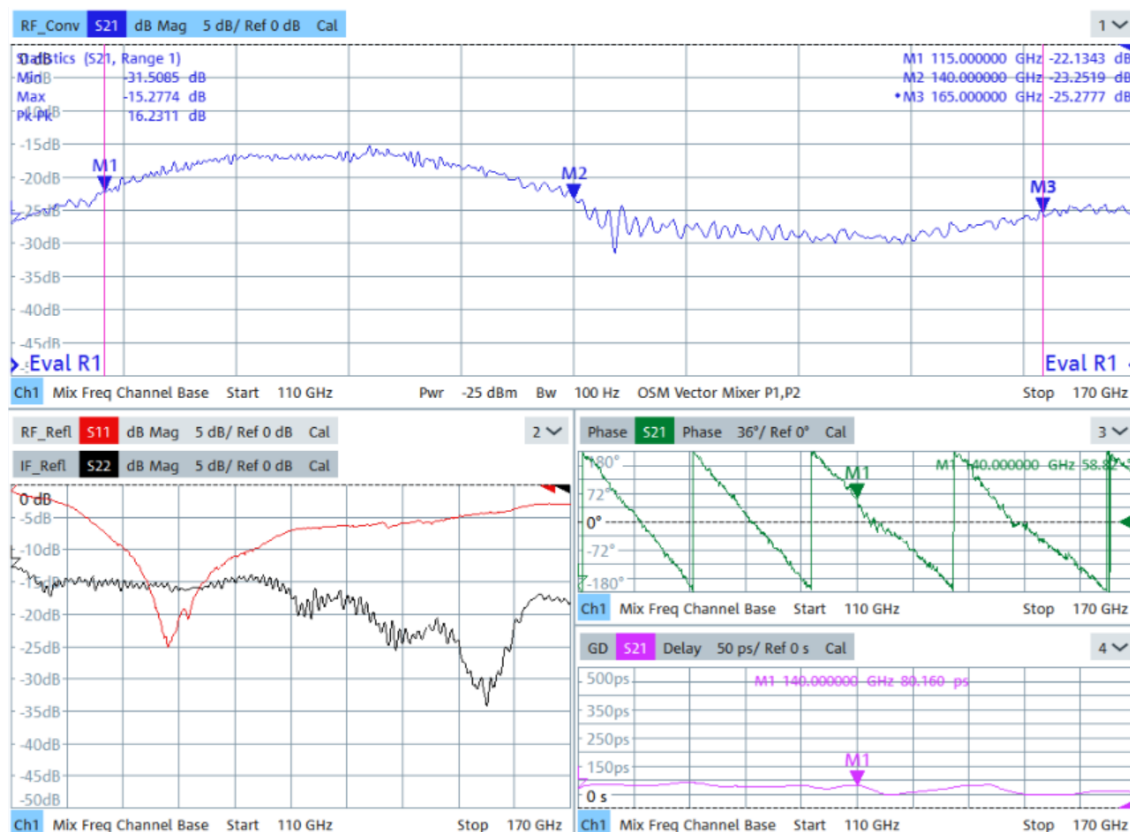
Fig. 23: D-band mixer measured with vector mixer calibration: Upper: Conversion loss, lower left: RF and IF port match, lower right: conversion phase and group delay
