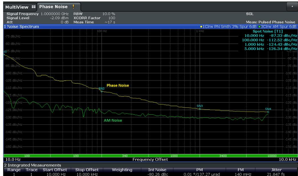
Figure 18, FSWP pulsed carrier noise measurement
