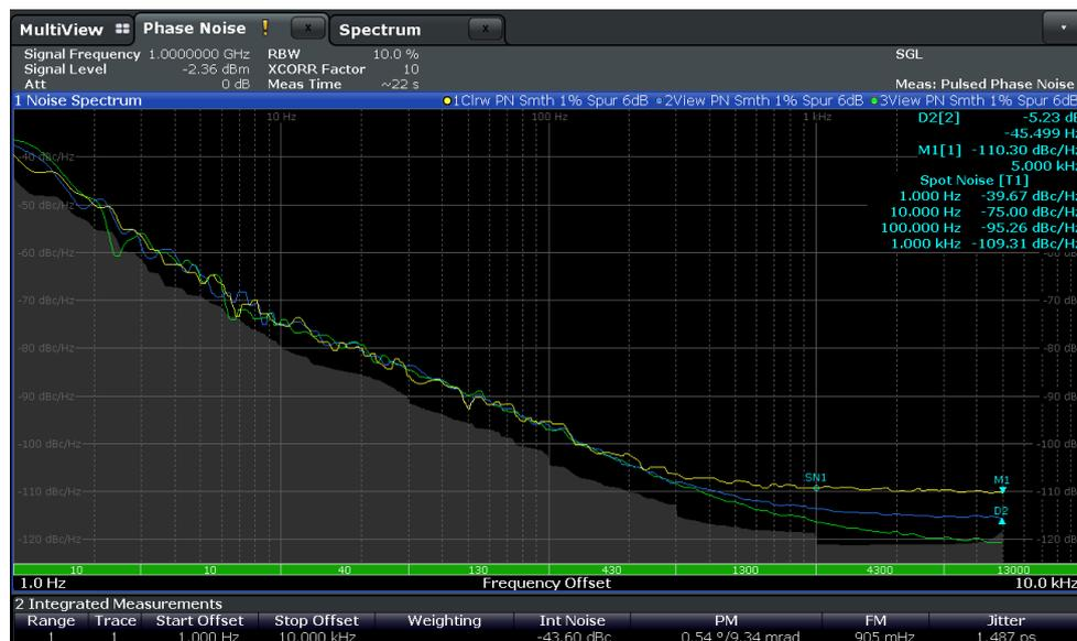
Figure 9, Differences in phase noise caused by changing pulse width
