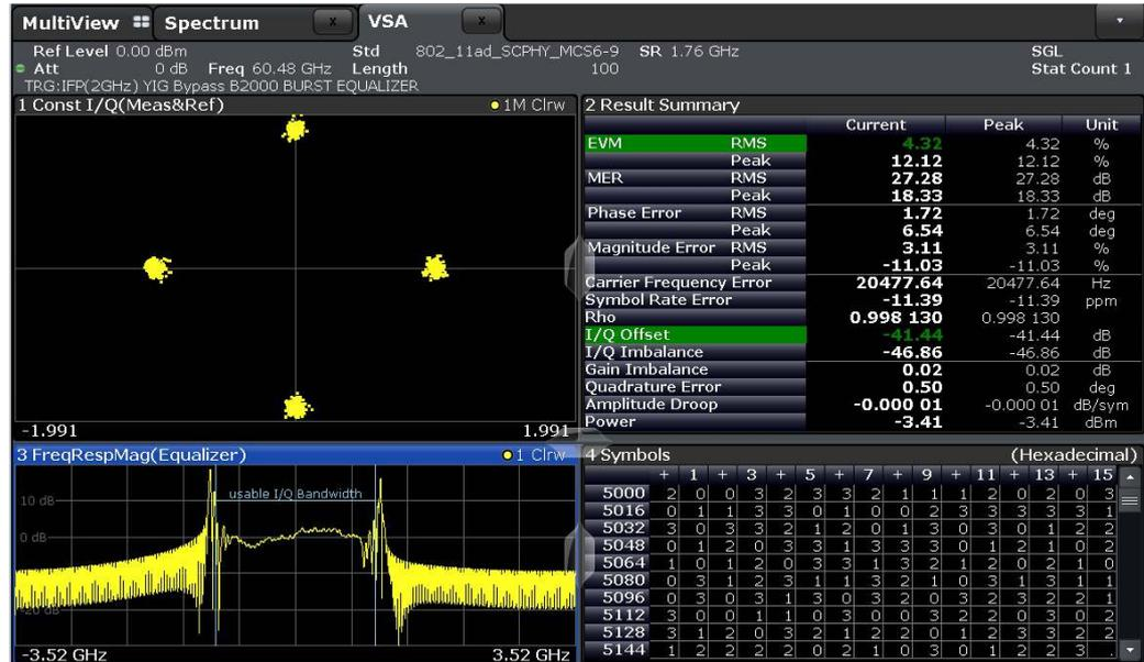
Figure 34: Example measurement result of equalized WLAN 802.11ad signal
