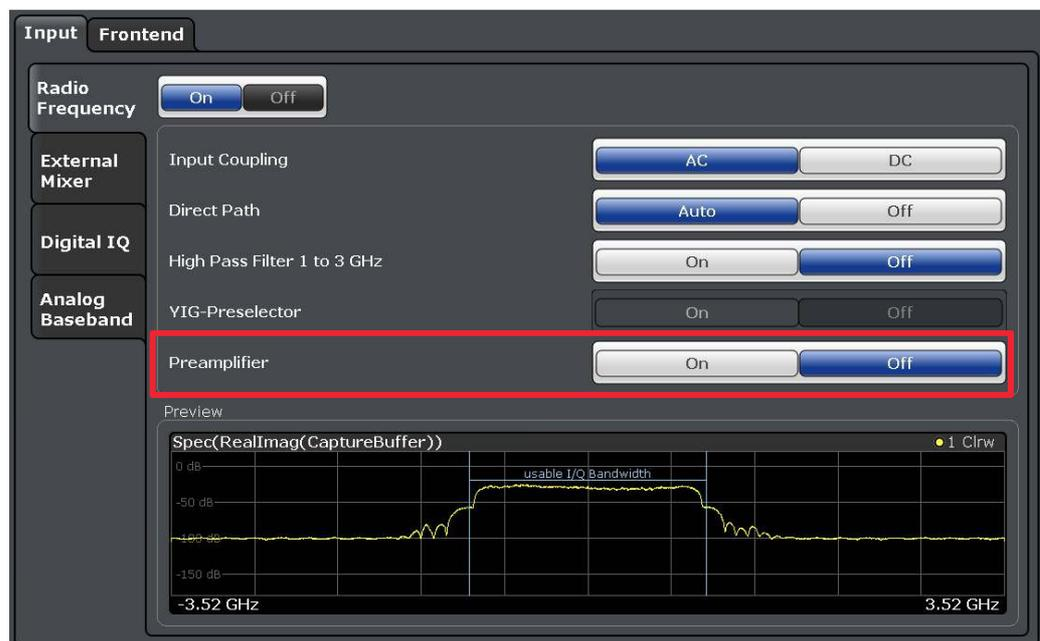
Figure 27: Activating Preamplifier in Input/Frontend dialogue
