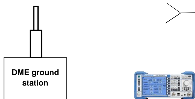
Fig. 11: Test setup for DME measurements in the field.
