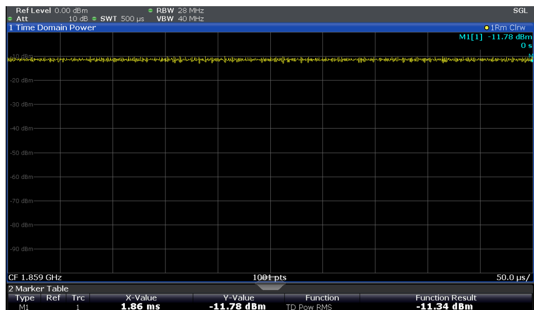
Fig. 3-7:Zero span measurement of a WCDMA signal with activated time domain power function
