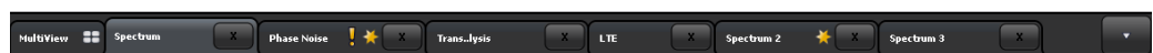
Fig. 3-15: Different channels allow different measurement configurations to coexist on the instrument. Tabs allow for quick changes between measurements.
