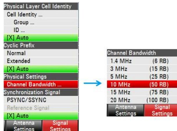
Fig. 6 LTE channel bandwidth configuration.
