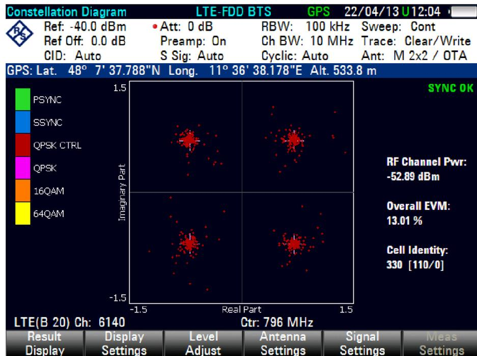
Fig. 10 LTE constellation diagram.
