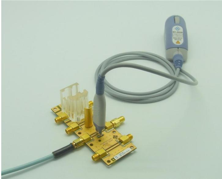
**Fig. 3-1: Probe test adapter used for performance evaluation**
