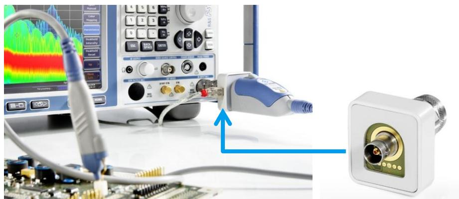
Fig. 2-3: Probe adapter RT-ZA9 connected to the R&S FSV spectrum analyzer
