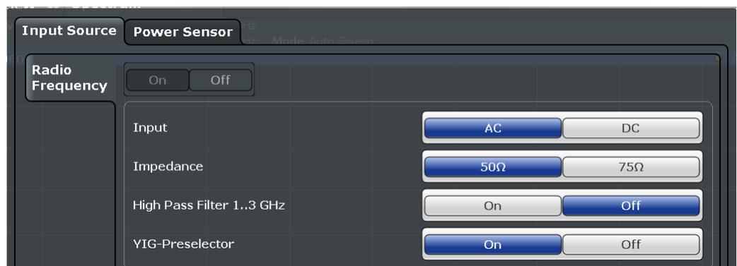
Figure 7: Input Source Dialog providing the High Pass Filter On/Off selection
