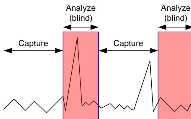
Fig. 1-1: Sequential capture and analysis as used in e.g. FFT analyzers
