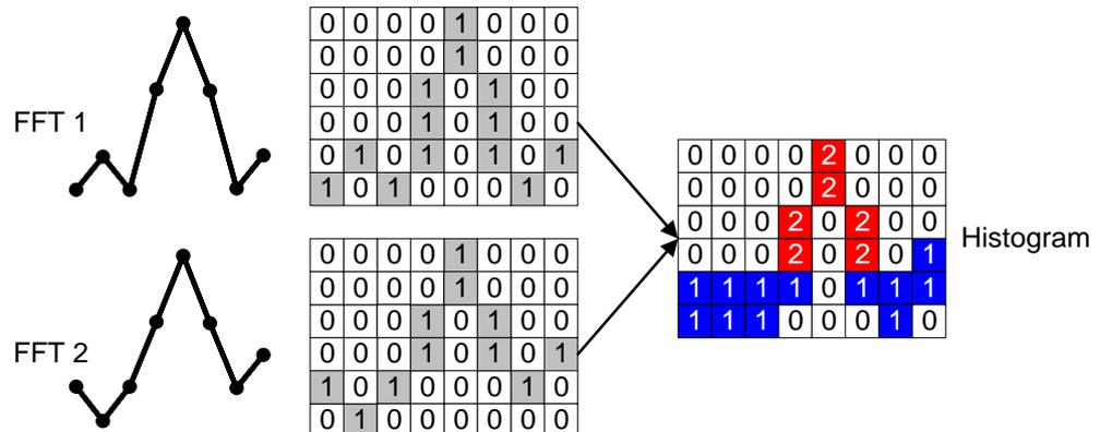
Fig. 4-9: Histogram calculation using vector style
