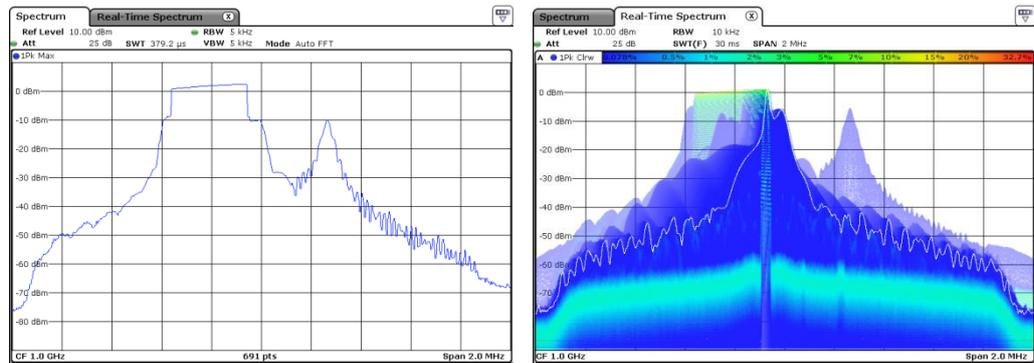
**Fig. 1-3: Comparison of a Max Hold spectrum analyzer trace and a persistence spectrum trace**
