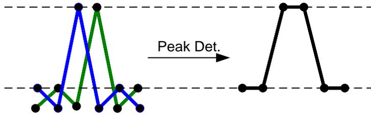
Fig. 4-2: Peak detector combining two FFTs into one spectrum
