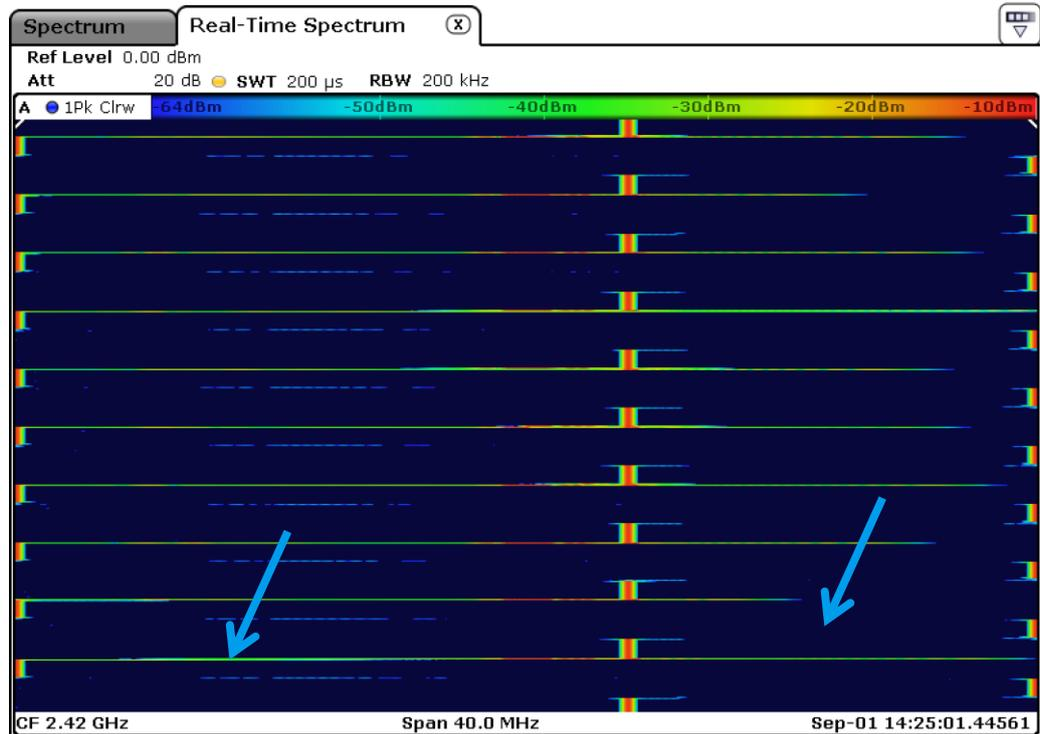
Fig. 4-1: Frequency hopper regularly hopping between 3 frequencies. First transition shows significant RF level, second transition shows almost no level during hop. Transitions highlighted by arrows.
