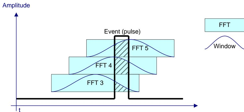
Fig. 2-7: Overlapping compensates effects resulting from windowing function
