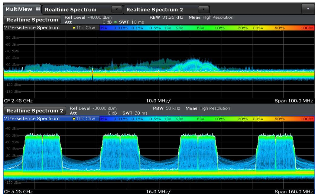
**Fig. 4-6: Frequency agile DUT in the 2.4 GHz ISM band and 5 GHz band. Persistence shows signal longer than its duration**
