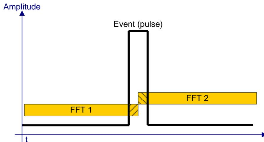
**Fig. 2-5: Pulse captured by two consecutive FFT time frames without overlapping**
