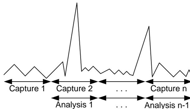
Fig. 1-2: Parallel capture and analysis as used in real-time analyzers
