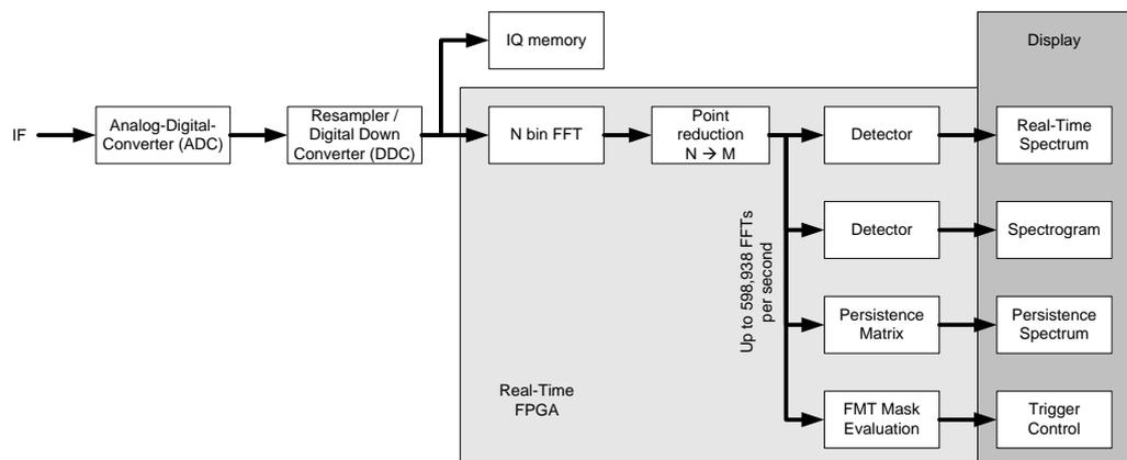
**Fig. 2-1: Signal flow chart of the digital real-time part of the Rohde & Schwarz real-time analyzers**
