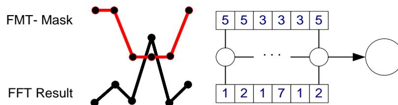
Fig. 3-3: Element-wise comparison of FMT mask with current FFT result
