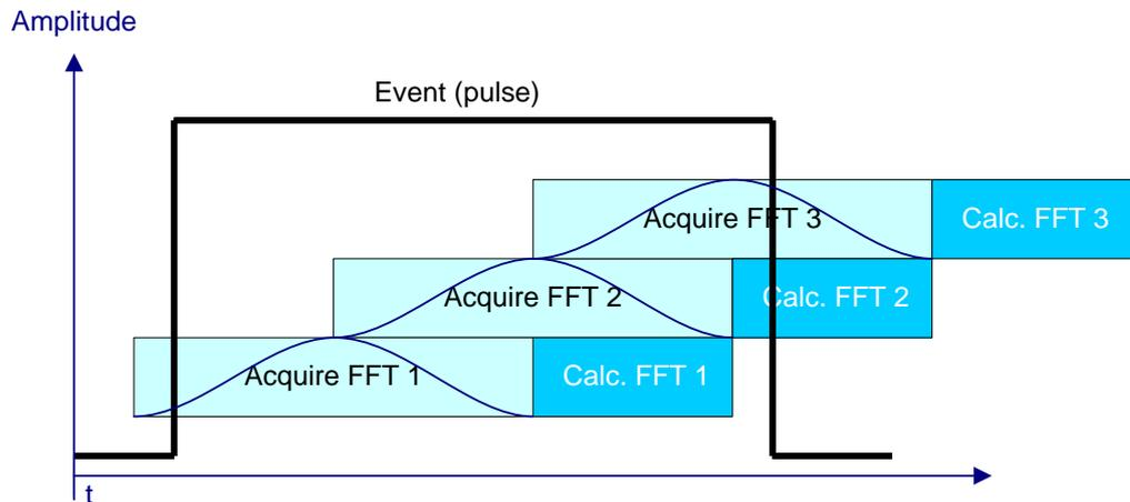
**Fig. 2-10: Real-time configuration with overlap; the measured event is longer than the POI time and therefore displayed with 100% true power**
