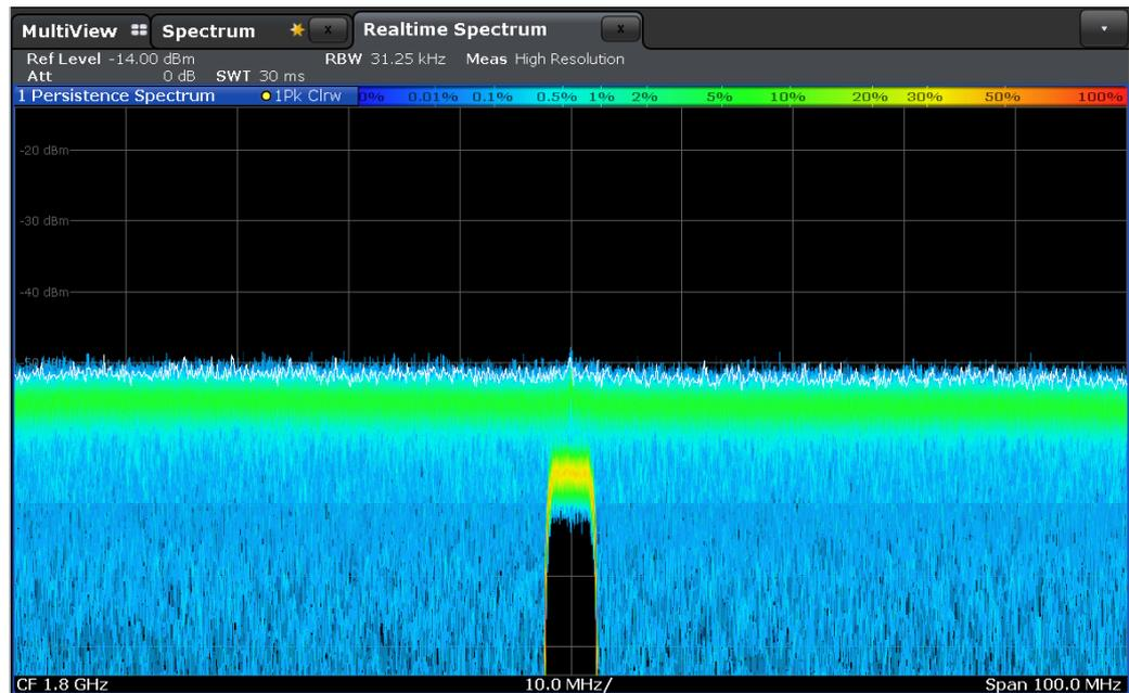
Fig. 4-7: Wideband noise-like signal covering a WCDMA signal
