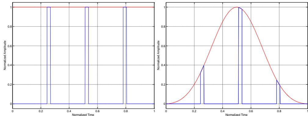
**Fig. 2-3: Pulse signal in time domain. Different window functions are applied to the same signal: left - rectangular - no weighting, right - Blackman - pulses on the right and left are highly attenuated**
