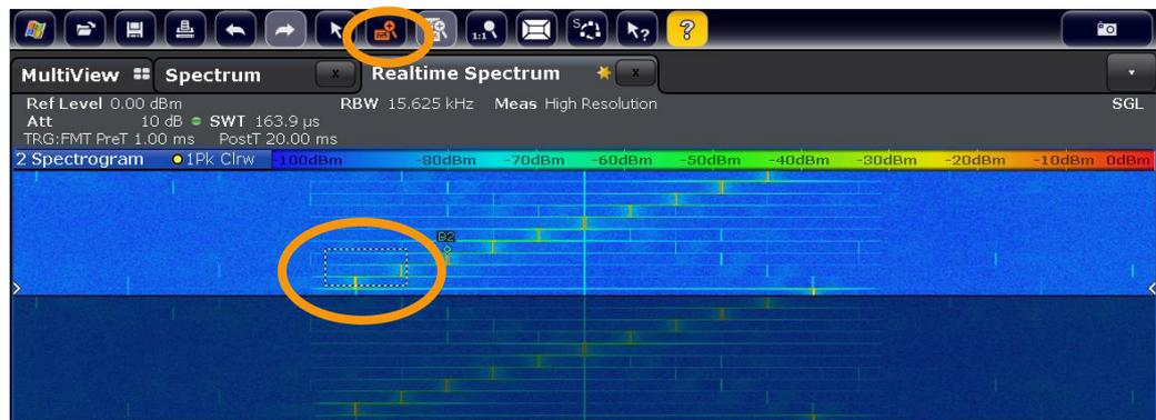
Fig. 2-12: Spectrogram with magnifying tool selected. Light area in spectrogram indicates zoom able area, dark area: not zoom able
