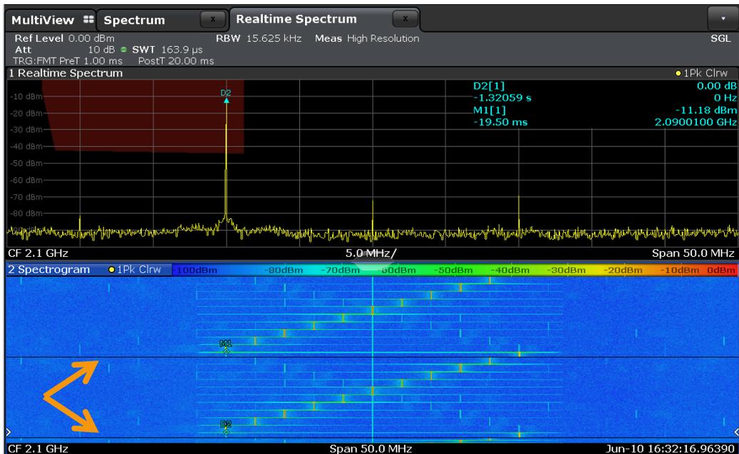
Fig. 4-3: Spectrogram with two black lines, indicating non-contiguous captures, i.e. gaps, due to triggered mode or single sweep operation
