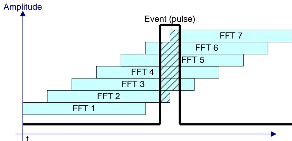
**Fig. 2-6: Pulse captured with several consecutive overlapping FFT time frames**
