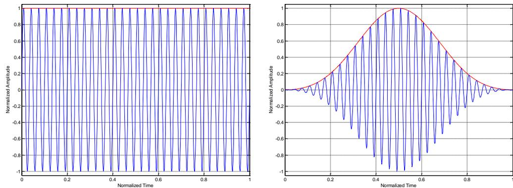
**Fig. 2-2: Sine wave signal in time domain. Different window functions are applied to the same signal: left - rectangular, right - Blackman**
