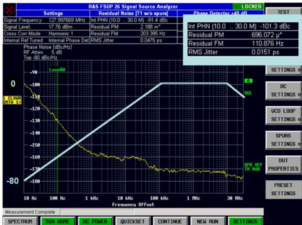
Figure 12: The RMS jitter calculated over the whole frequency offset range gives 0.0475ps. When the transducer factor (figure 11) is applied, which is illustrated in the picture as blue line, the result changes to 0.0151ps.
