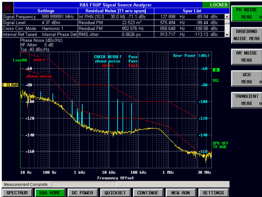
Fig. 10: Test result of limit lines: The random jitter passes the test, whereas periodic jitter is above the limit.
