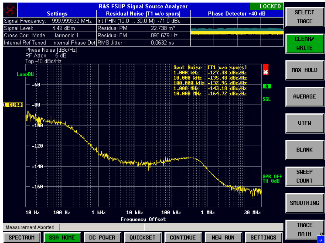
Fig. 3: Phase noise measurement of a high-end DUT.
