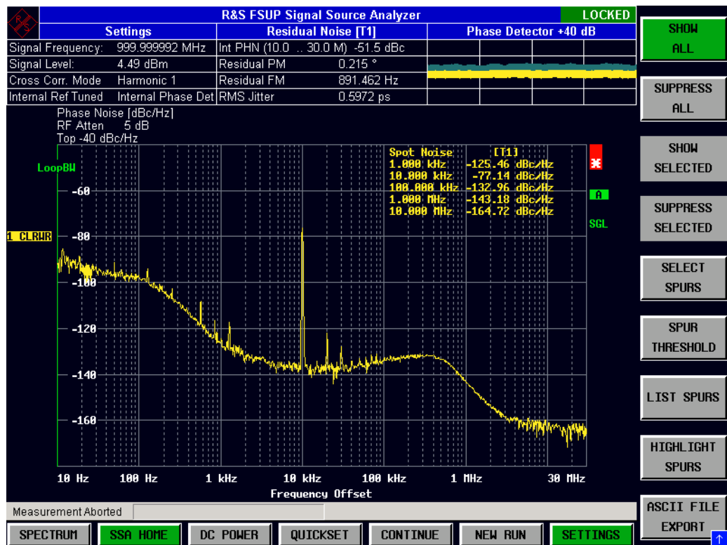
Fig. 4: Same measurement as in Fig. 3 with "SHOW ALL" selected in the spur setting menu.
