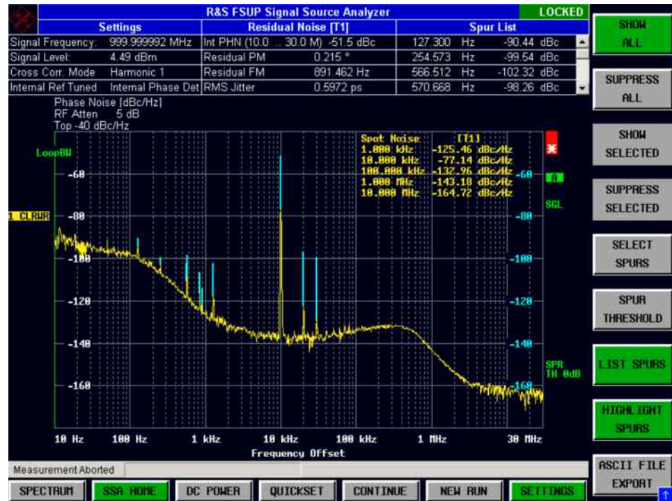
Fig. 5: Same measurement as in Fig. 3 with “LIST SPURS” and “HIGHLIGHT SPURS” selected in the spur setting menu.
