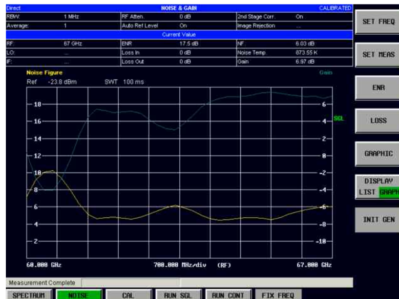
Figure 5: The screen shot displays an example amplifier NF measurement using a DUT designed for W-band applications. The blue trace shows the amplifier gain and the yellow trace is amplifier noise figure.
