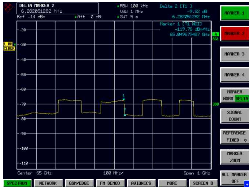
Figure 3: Noise Floor measured with spectrum analyzer R&S FSU67, where ENR output is pulsed on and off.
