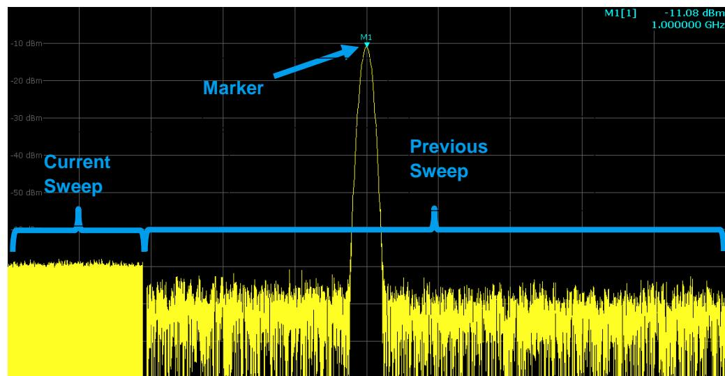
If the test software reads the trace data under such conditions, the resulting array of values consists of a mixture from two subsequent measurements. The data is obviously invalid.
