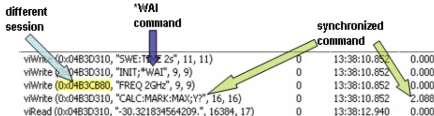
Note that **\*WAI** does not affect the communication with other instruments. In the example above, the frequency setting of a second instrument is performed immediately after the initiation of the sweep. The marker search operation however, is delayed for 2 seconds, because the sweep time was set to this value.
