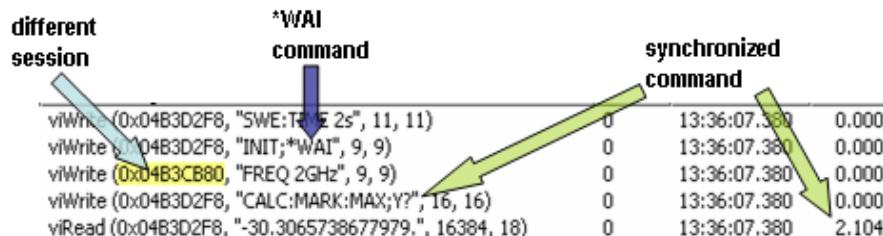
Important is the fact that the result of the synchronized operation (here marker value) is returned upon completion of the preceding commands (here sweep completed).
