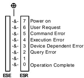
Synchronization can be achieved by polling the status of the Operation Complete bit using the query command `*ESR?`. A read operation on the Event Status Register is destructive, i.e. the register is cleared after the read operation and thus the contents cannot be retrieved multiple times.
