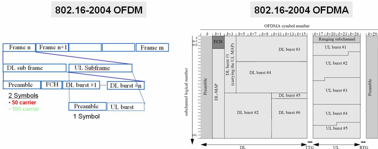
Figure 1: Comparison of frame structure of 802.16-2004 OFDM system and 802.16-2004 OFDMA. In OFDM e.g. the downlink consists of a preamble followed by an FCH field and the bursts for the different subscribers. In OFDMA mode the bursts are allocated according to downlink map.
