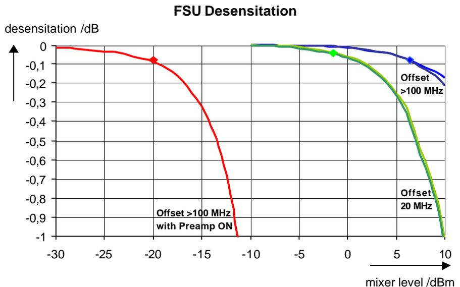
Fig. 3 Desensitization of a -40 dBm CW signal dependent on the level and offset of a WCDMA down-link signal (crest factor ~ 10.5 dB)
