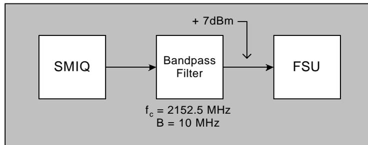
Fig. 9 Test setup for the measurement examples
