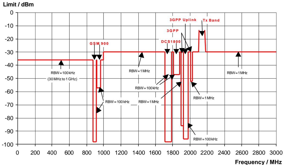
Fig. 1 Limits for spurious emissions in the Frequency range up to 3 GHz.
