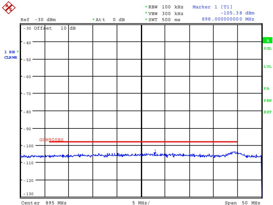
Fig 16 Spurious emission measurement in the GSM900 band.
