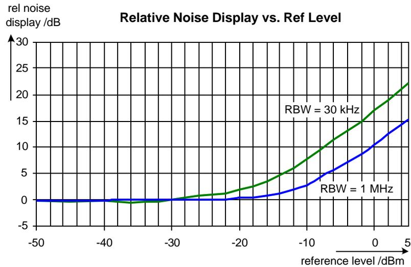
Fig. 5 Inherent noise floor of the FSU dependent on the reference level (reference is -30 dBm reference level)
