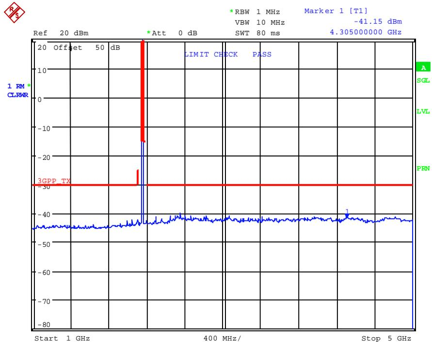
Fig 17 Spurious emission measurement in the 1 to 5 GHz band.
