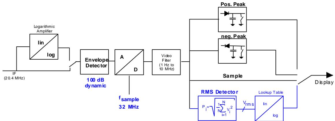
Fig. 6 Block diagram of the detectors in the FSU spectrum analyzer family.
