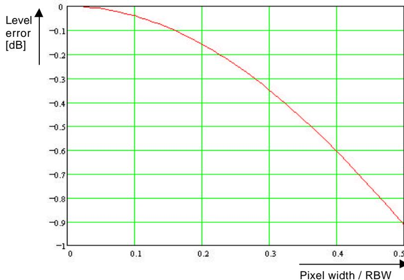
Fig 8 Level error depending on the pixel width / RBW ratio
