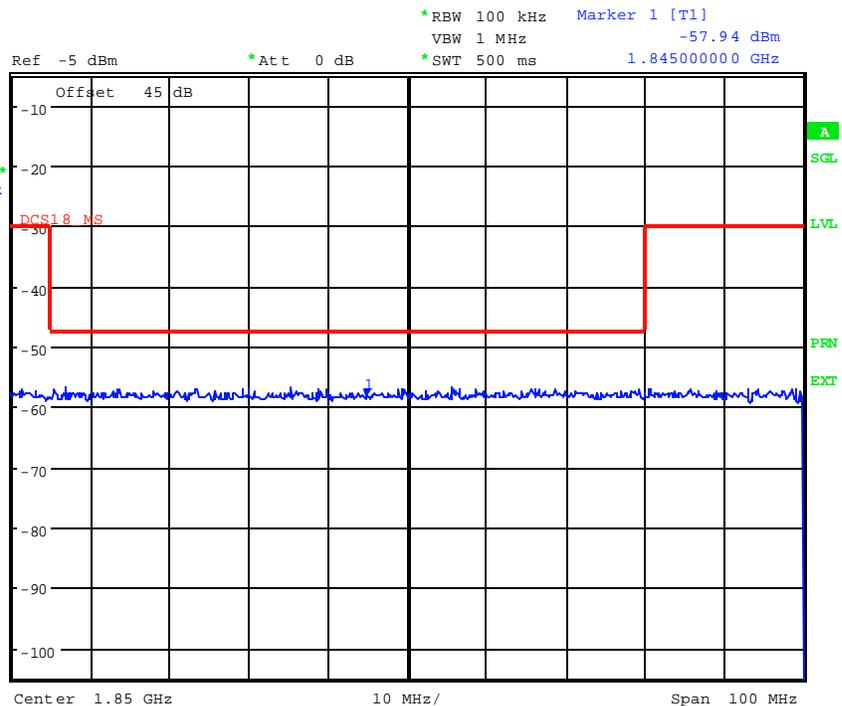
Fig 14 Spurious emission measurement in the DCS 1800 MS band.
