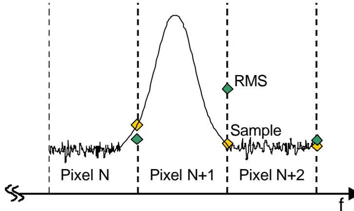
Fig 7 Illustration of sample and RMS results in a pixel
