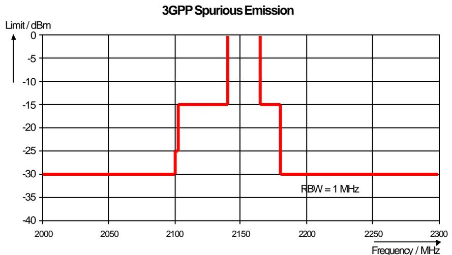
Fig 10 Spurious emissions close to the 3GPP transmit band (BTS transmit frequency = 2152.5 MHz)
