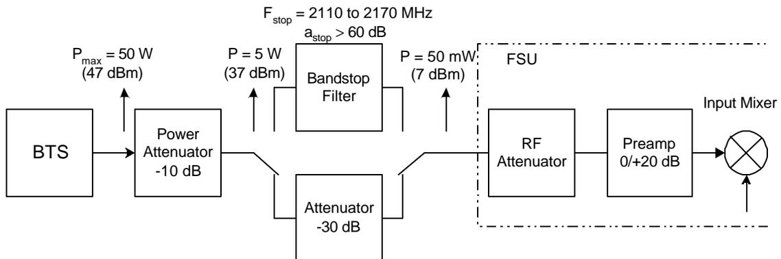
Fig. 18 Diagram of a test setup for spurious emission measurements.
