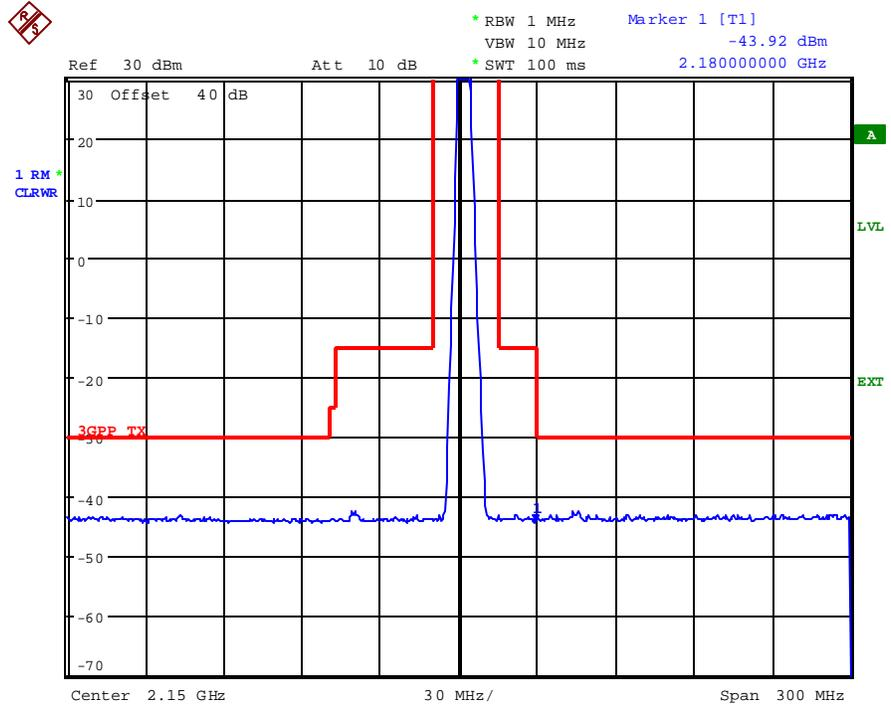
Fig 12 Spurious emission measurement close to the TX band.
