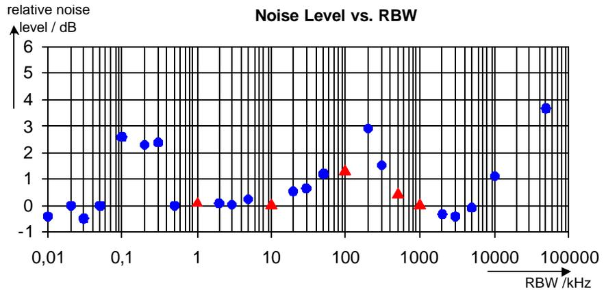
Fig. 4 Inherent noise floor of the FSU dependent on the resolution bandwidth (reference is 10 kHz RBW)
