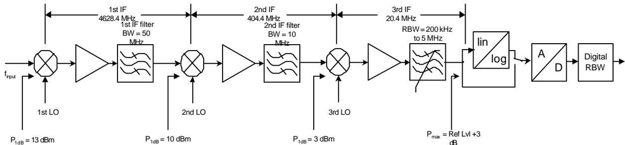
Fig 2 Simplified FSU RF block diagram
