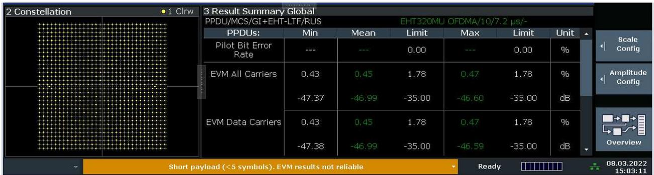
Short Payload warning for signals with less than 5 symbols
