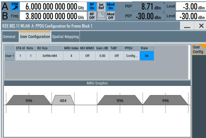
Signal setup with punctured 40MHz block
