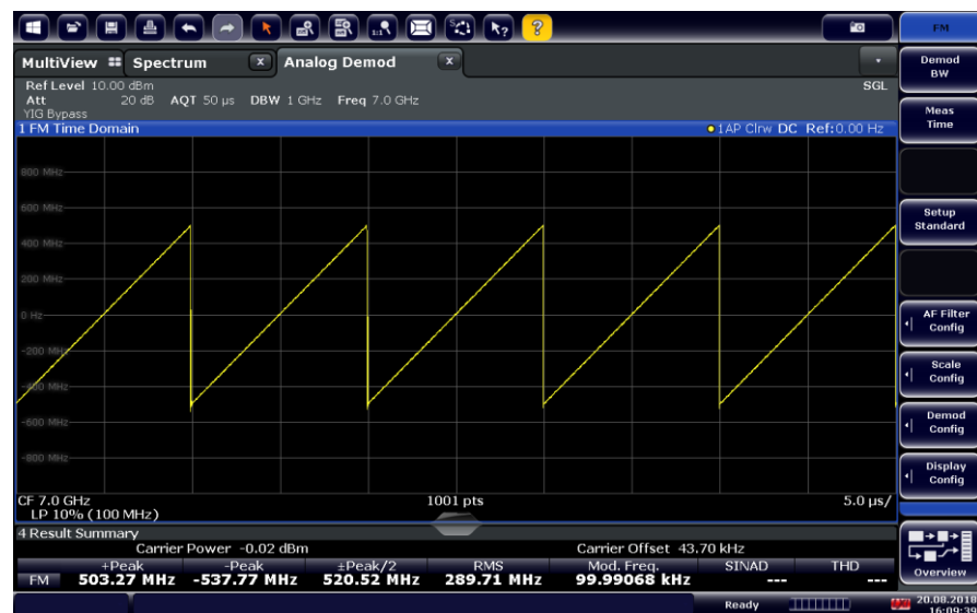
Figure 1: Demodulated chirp signal showing frequency deviation and chirp length
