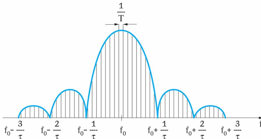
Figure 1: Typical display of a pulse signal spectrum showing pulse width  $\tau$  and pulse interval  $T$
