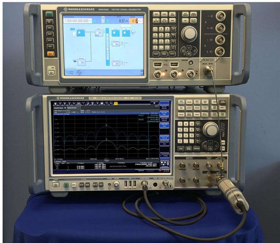
Figure 3: Picture of the test setup for pulsed measurements
