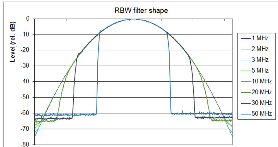
Fig. 8: Normalized RBW shape for the range from 1 MHz to 50 MHz
