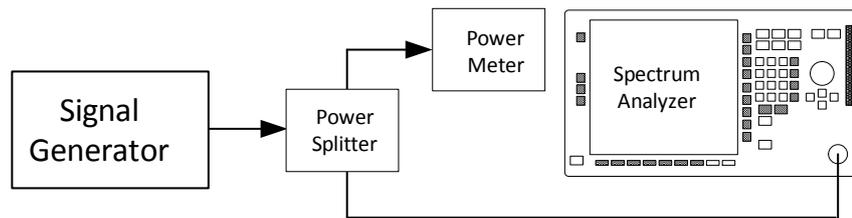
Figure 2: Test setup for pulsed measurements
