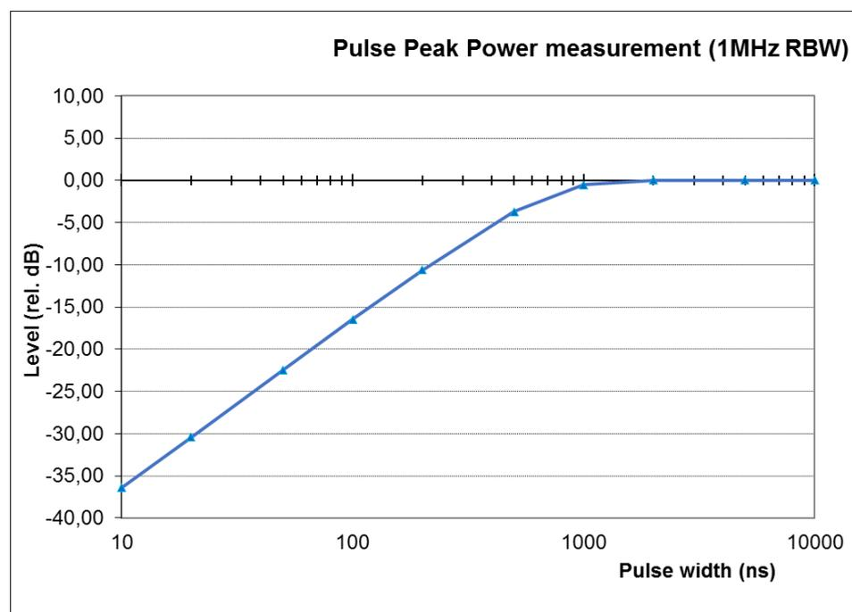
Fig. 6: Pulse peak power reading versus pulse length for 1 MHz RBW setting
