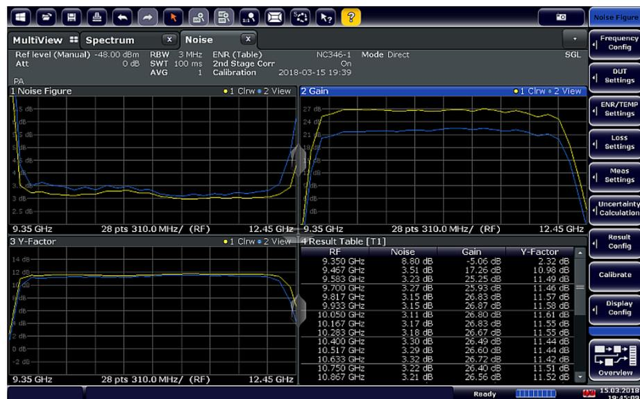
Fig. 4: Test result of pulsed amplifier (yellow: gated sweep, blue: continuous sweep)
