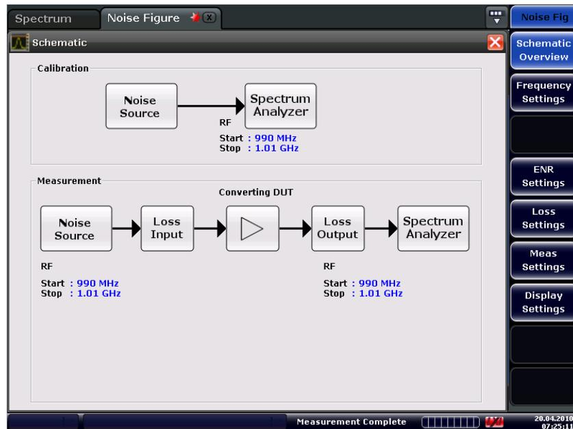
Figure 1: Configuration window for making noise figure measurements
