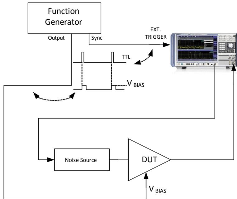
Figure 2: Test setup for pulsed noise figure measurements
