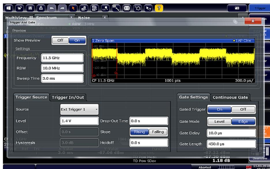
Fig. 3: Trigger and Gate configuration dialog
