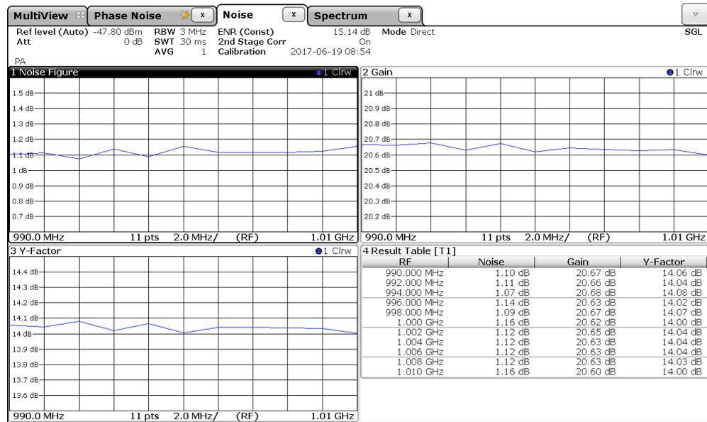
Fig. 3-3: FSWP-K30 Noise Figure Measurement of Test Amplifier
