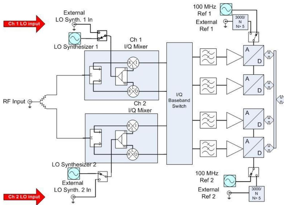
**Fig. 2-7: FSWP Block Diagram, Showing External LO Inputs**
