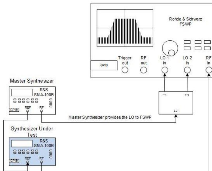
**Fig. 3-19: Setup for measuring the Residual Noise of a Frequency Synthesizer**
