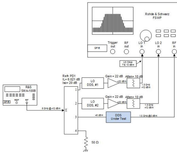
Fig. 3-17: Residual Noise Measurement Setup for a DDS
