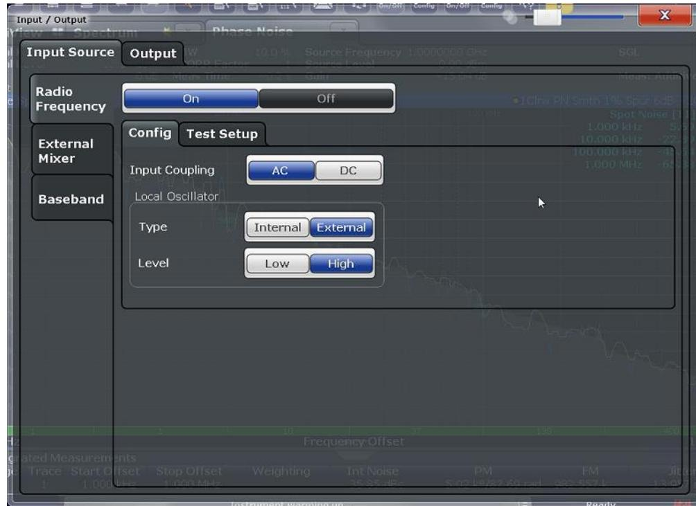
**Fig. 3-8: FSWP External LO Control Setup**
