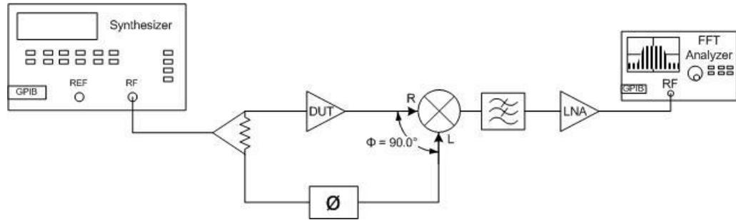
Fig. 1-6: Residual Phase Noise Measurement, Using a Double-Balanced Mixer as a Phase Detector
