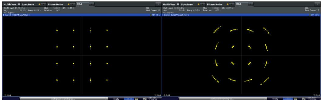
**Fig. 1-1: Effect of Phase Noise on a 16-QAM Constellation**
