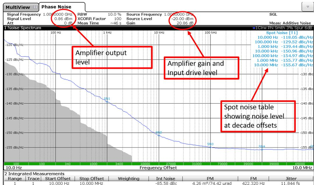
**Fig. 3-2: Amplifier Residual Phase Noise Measurement**
