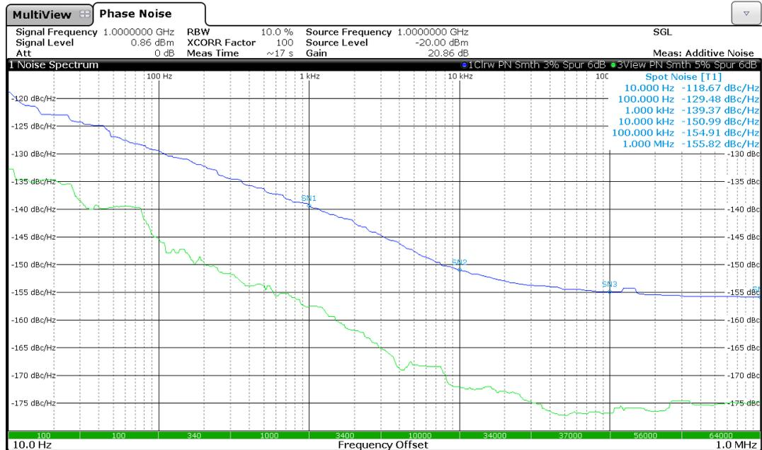
**Fig. 3-5: Amplifier Phase Noise and FSWP Noise Floor**
