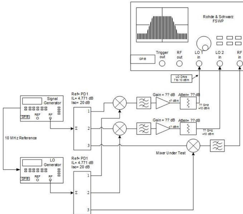
**Fig. 3-15: Three-Converter Residual Noise Setup Using a Shared LO**
