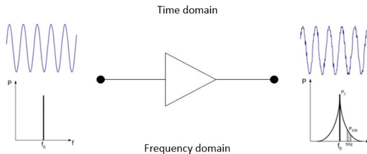
Fig. 1-2: Phase Noise of an Ideal vs. Real-world Signal
