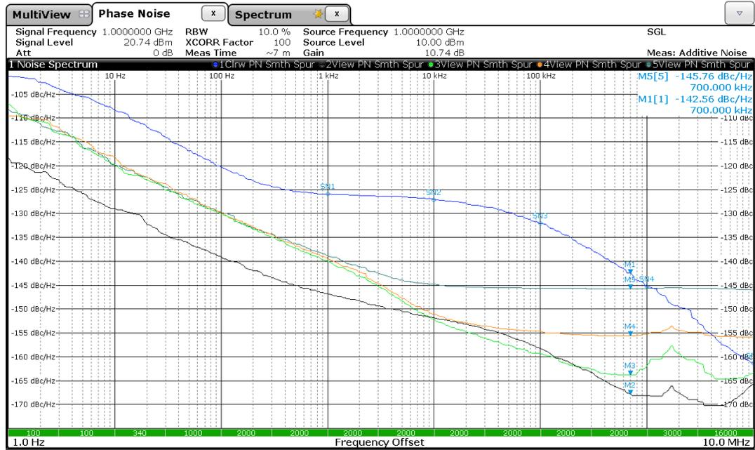
**Fig. 3-6: Residual Phase Noise of Amplifier at Various Drive Levels**
