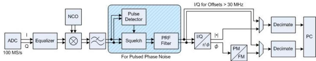
**Fig. 2-2: FSWP DSP for One Channel**
