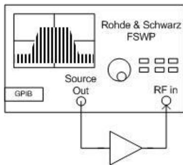
Fig. 3-1: FSWP DUT Connections for a Simple Residual Noise Measurement
