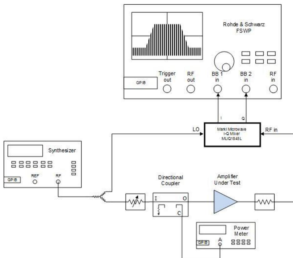
**Fig. 3-21: Amplifier Residual Noise Setup Using a Marki MLIQ-1845L Mixer**
