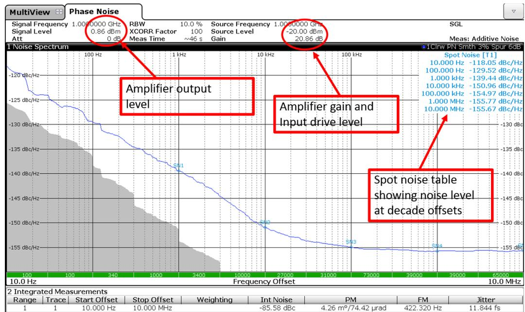
**Fig. 3-2: Amplifier Residual Phase Noise Measurement**
