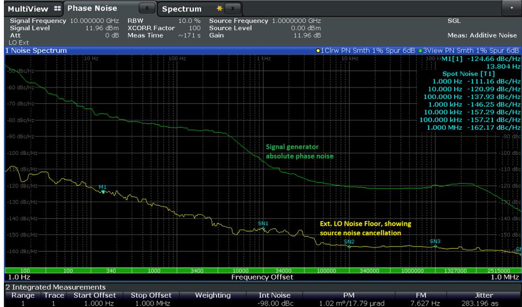
Fig. 3-10: FSWP Noise Floor Measurement, Using an External LO
