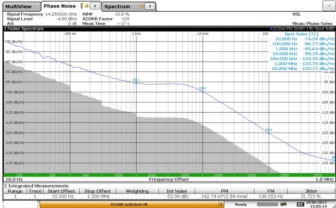
**Fig. 3-12: Phase Noise of a Ku-Band Satellite up Converter**
