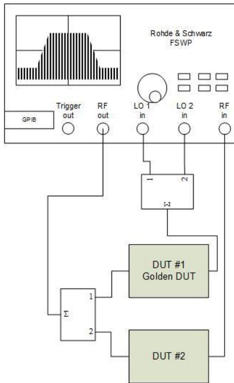
**Fig. 3-13: Setup for Two-Converter Method**
