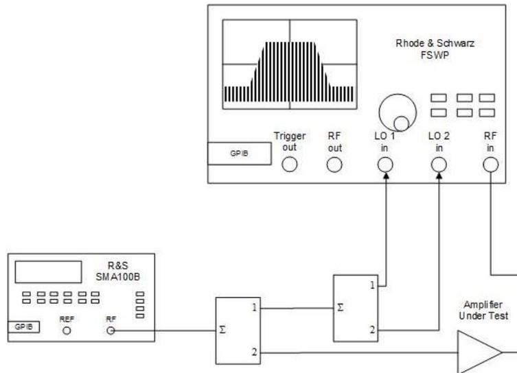
**Fig. 3-9: Simple Two-Port Residual Noise Measurement, Using an External Source**
