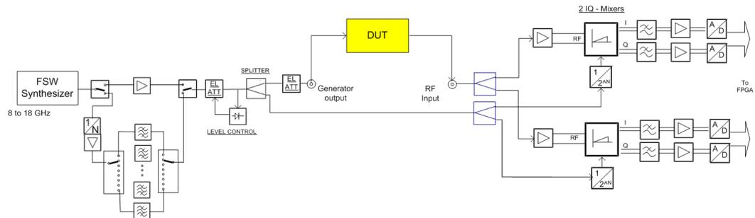
**Fig. 2-5: FSWP B64 Signal Source Block Diagram**
