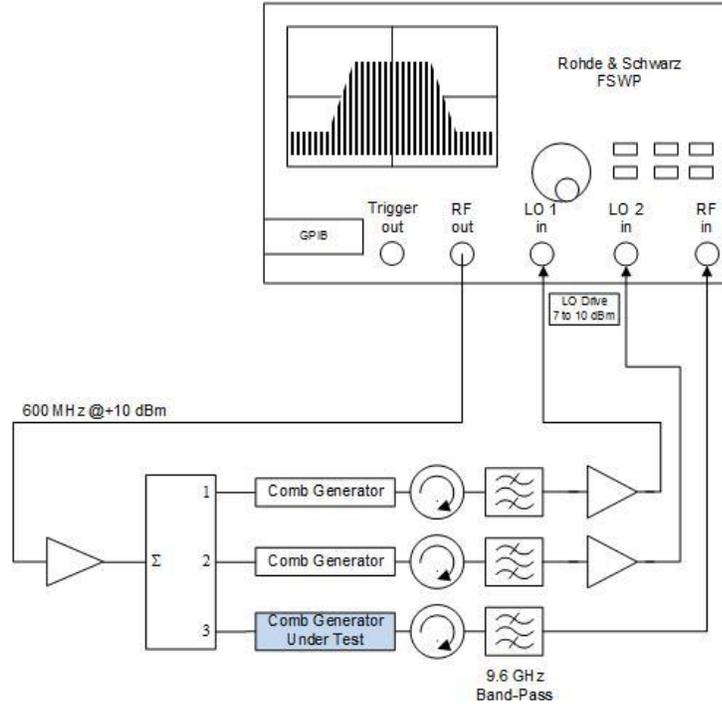
**Fig. 3-16: Residual Noise Setup for a Comb Generator**
