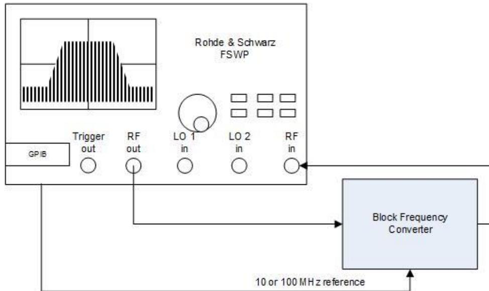
**Fig. 3-11: Phase Noise Measurement Setup for a Block Frequency Converter**
