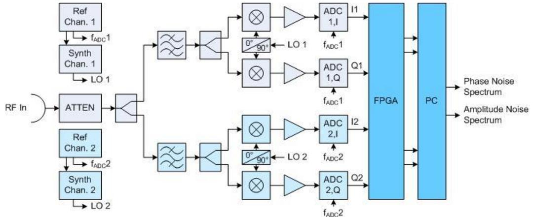
**Fig. 2-1: FSWP Analog Block Diagram**
