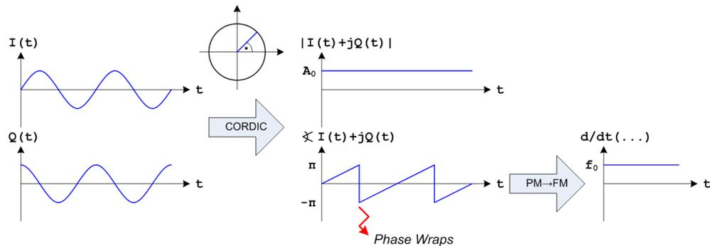
**Fig. 2-3: AM and FM Demodulation of a Carrier**
