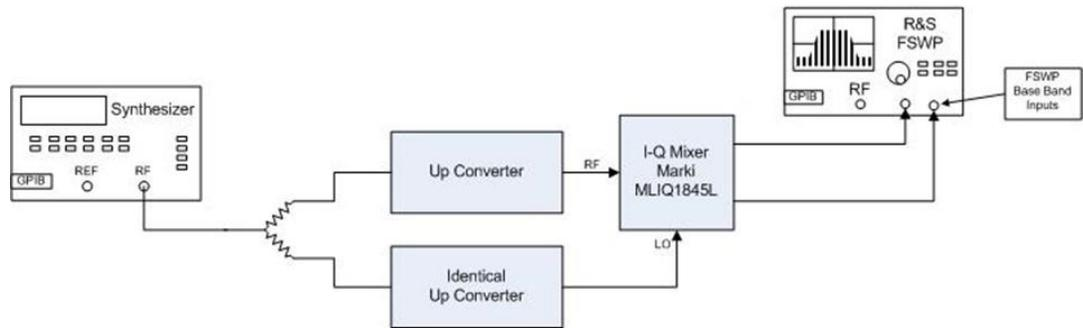
**Fig. 3-23: Frequency Converter Residual Phase Noise, Using an External Mixer**
