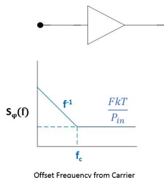
Fig. 1-5: Two Phase Noise Components of an Amplifier
