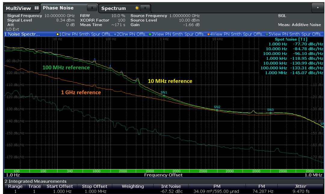
**Fig. 3-20: Residual Phase Noise of R&S SMA100 Signal Generator**
