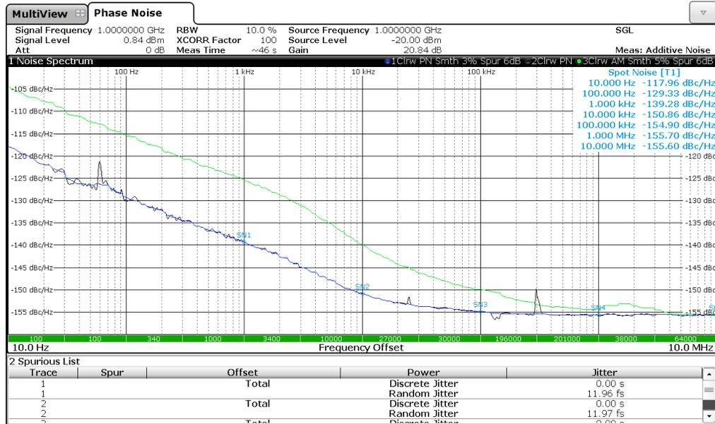
**Fig. 3-4: Residual Noise Measurement Showing AM Noise and Spurs**
