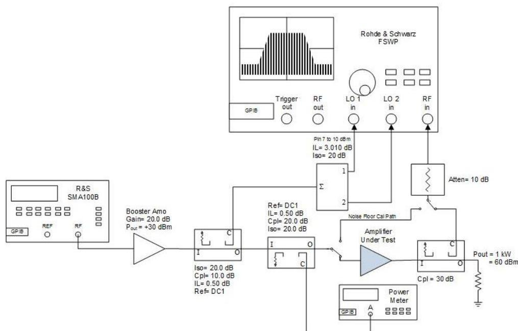
**Fig. 3-7: Residual Noise Measurement Setup, Using an External Booster Amplifier**
