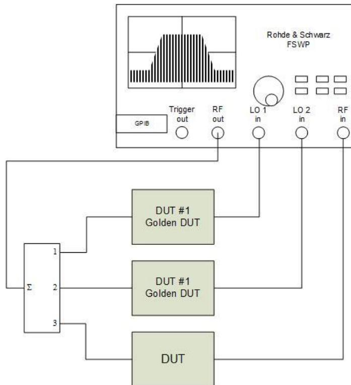
**Fig. 3-14: Setup for the Three-Converter Method**
