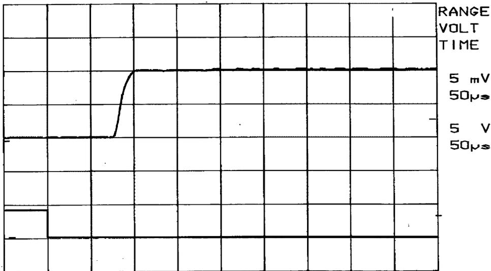
**FIG. 4: Transient response of FMA/B FM demodulator**
