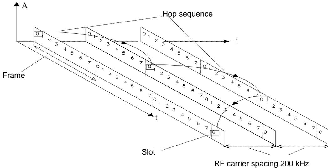
**FIG. 2: Frequency hopping mode**
