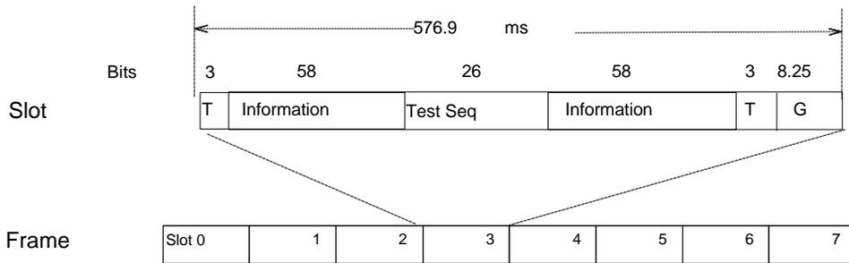
**FIG. 1: Time slot and frame**
