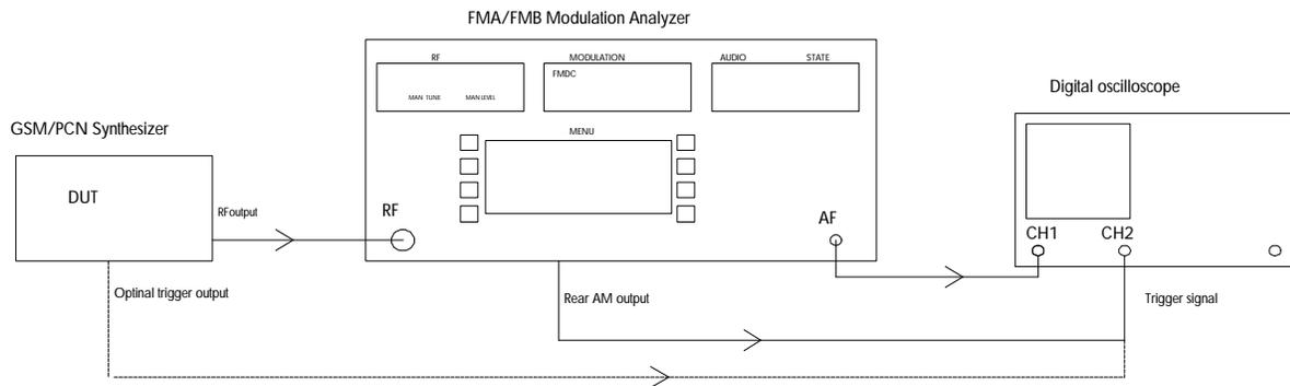
**FIG. 3: Test setup for transient measurements**
