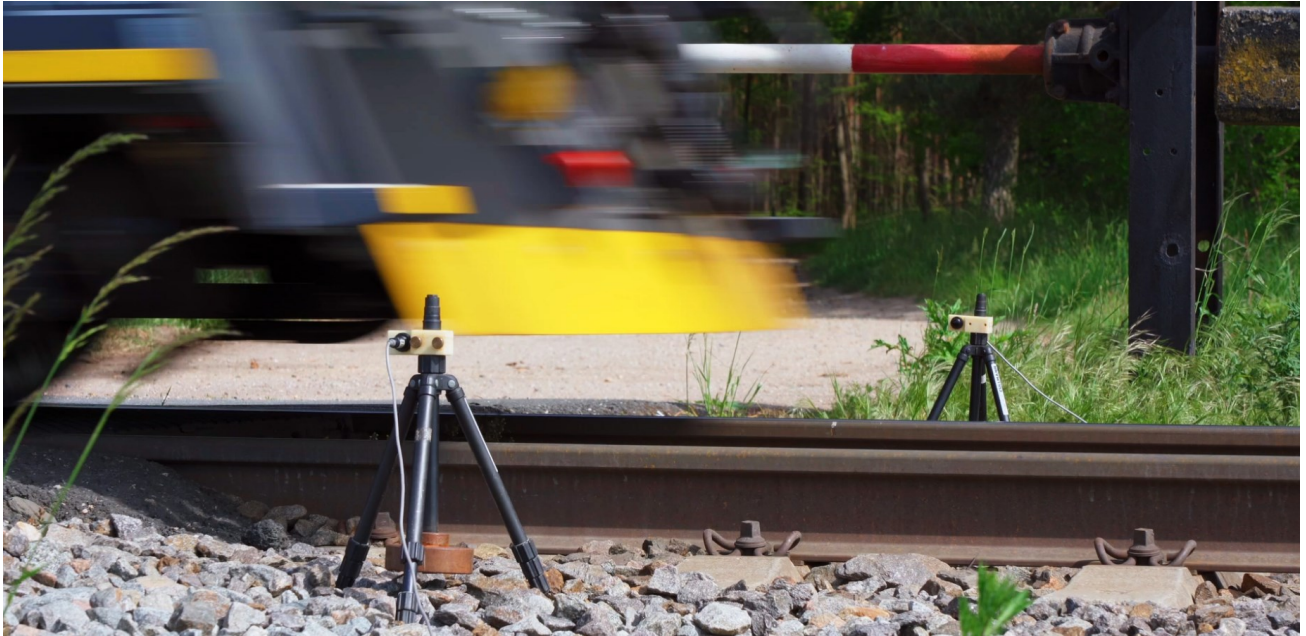
Figure 5 Start of measurement triggered using a light barrier.
