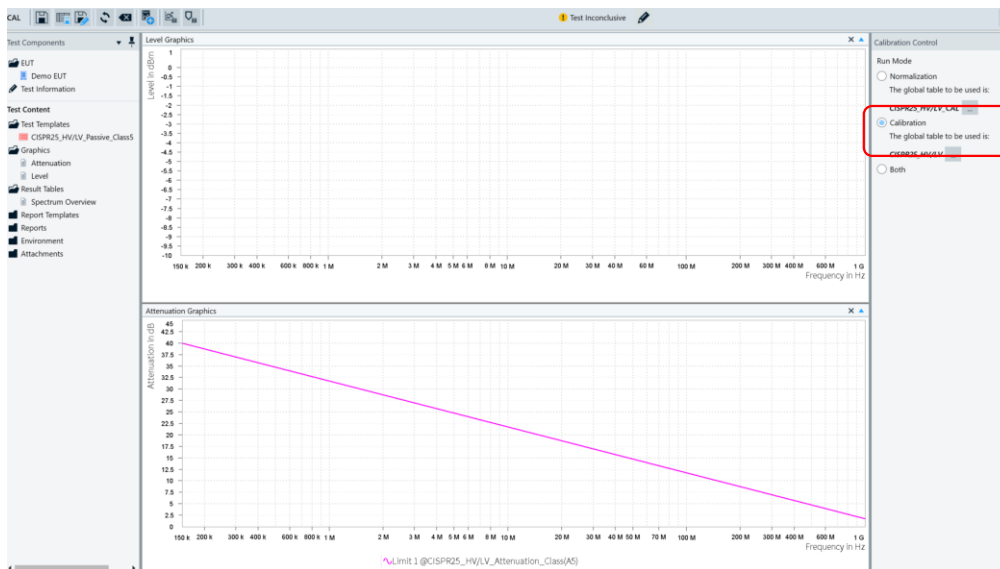
Figure 4: Coupling attenuation measurement test view.
