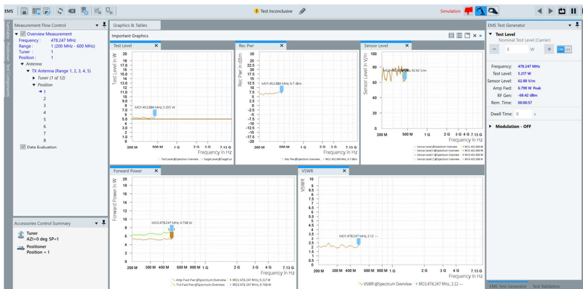
Figure 7 Unloaded test view during mode-tuned measurement.
