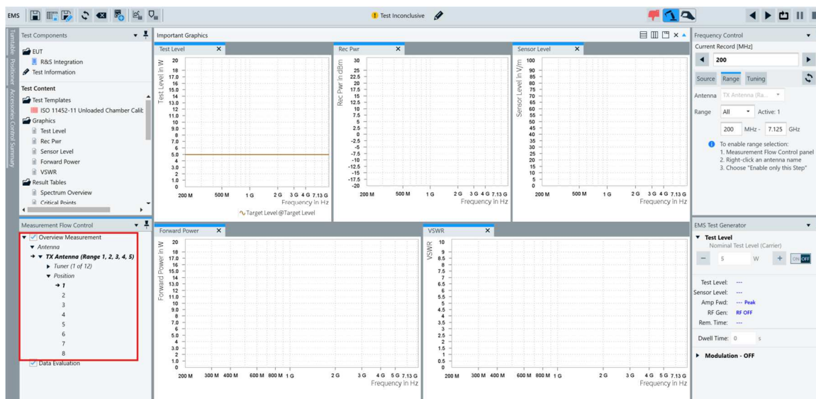
Figure 5 Unloaded chamber test view for mode-tuned test.
