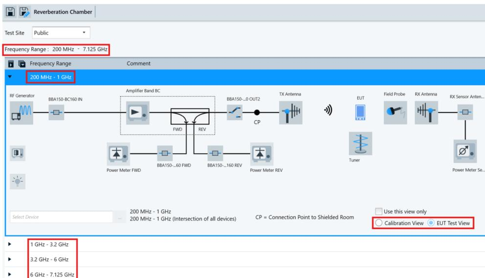
Figure 4 EUT View (200 MHz – 7.125 GHz) of Hardware Setup
