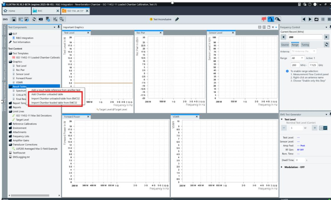
Figure 12 Selection of unloaded chamber calibration results inside the test
