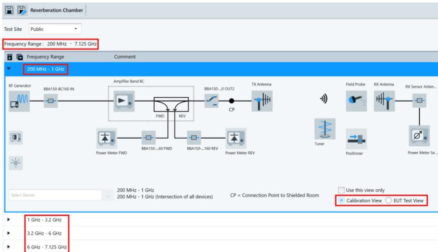
Figure 3 Calibration View (200 MHz – 7.125 GHz) of Hardware Setup
