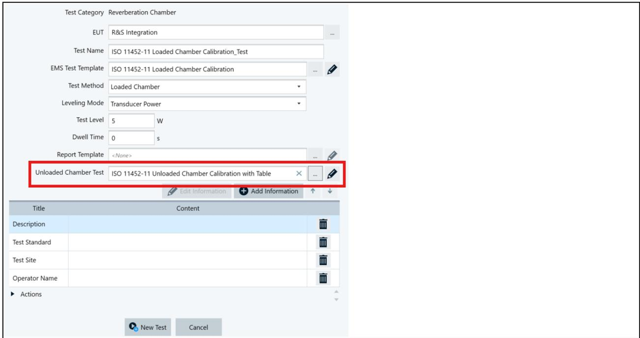
Figure 11 Test Application Setting View to select the unloaded chamber calibration result table
