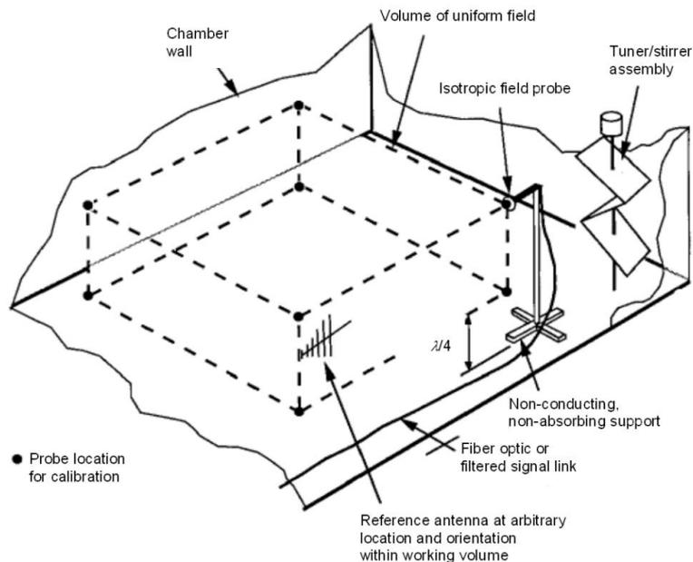
Figure 1 Test volume in RVC, SOURCE: IEC 61000-4-21 [1]
