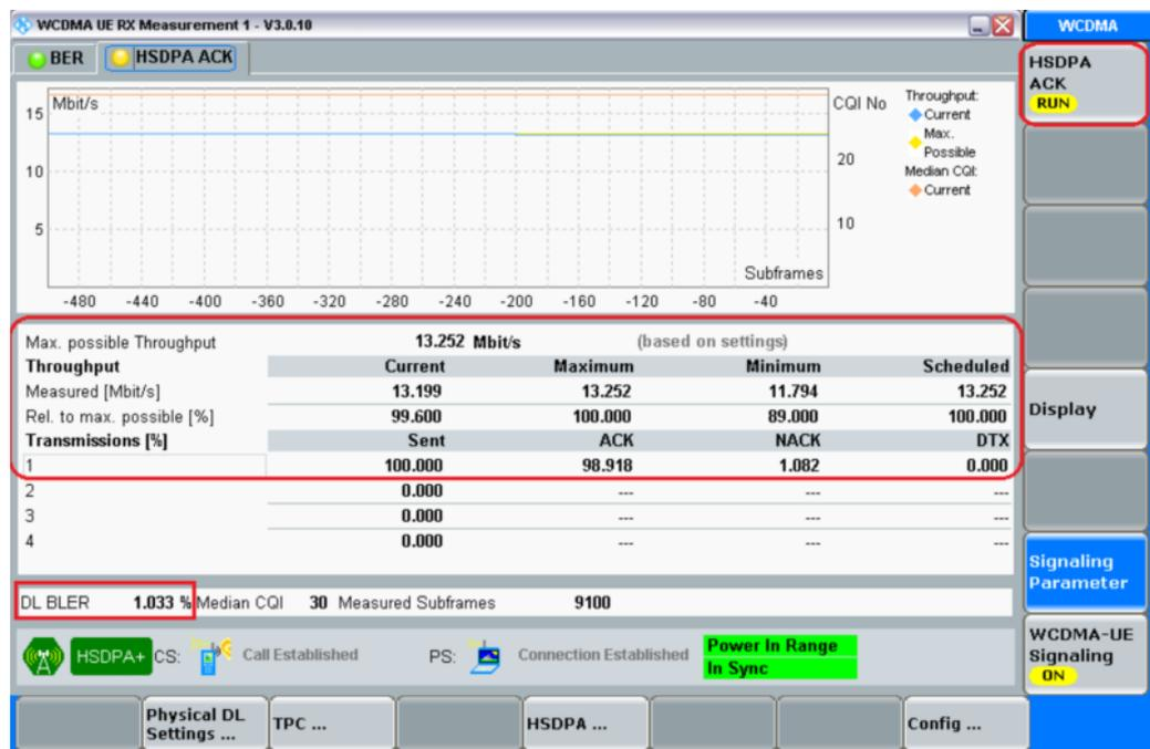
Fig. 42: Maximum input level for HS-PDSCH reception (64QAM).
