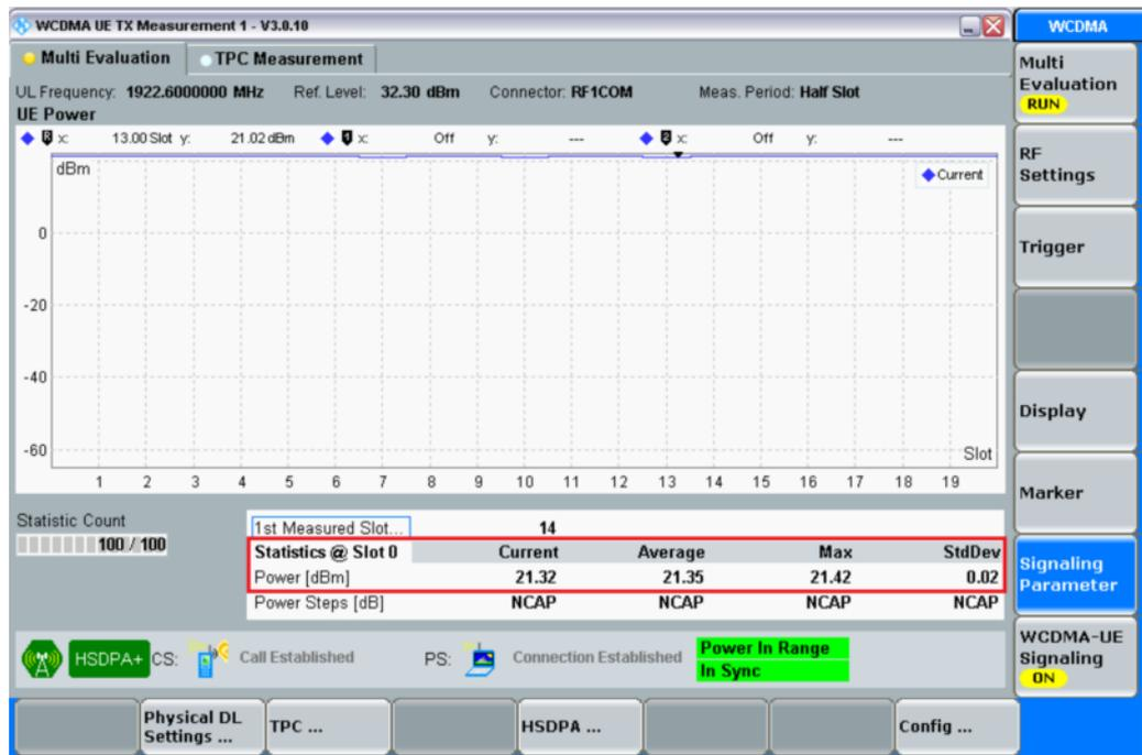
Fig. 16: Maximum output power with HS-DPCCH measurement results.
