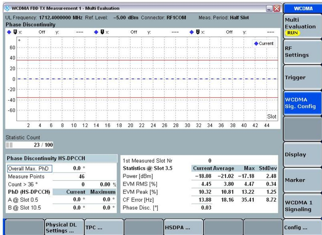
Fig. 36: The EVM and phase discontinuity with HS-DPCCH measurement results.
