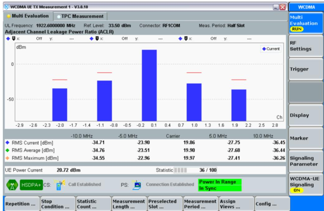
**Fig. 30: ACLR with HS-DPCCH measurement results.**
