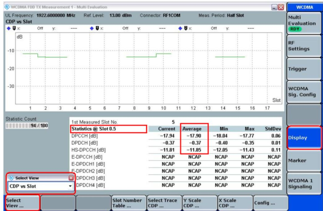
Fig. 20: Measurement results for the relative code-domain power.
