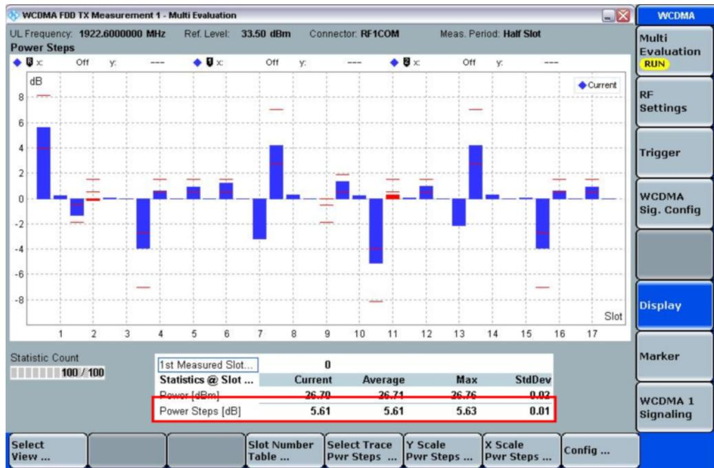
Fig. 186: Power step measurement around Measurement Point 1 for TPC\_cmd=1.
