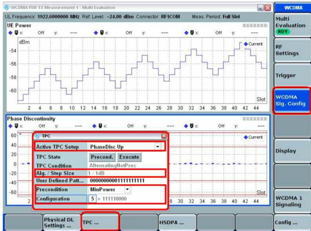
Fig. 33: Configuring a "phase discontinuity up" measurement.
