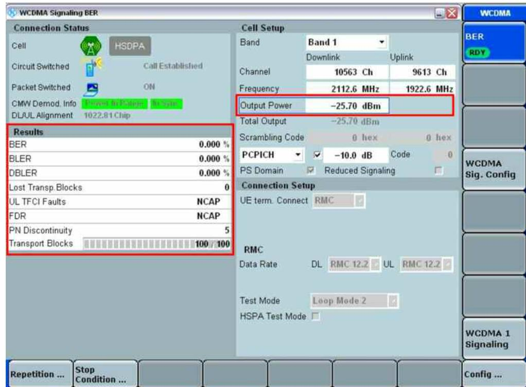
Fig. 40: BER results for the maximum input level.
