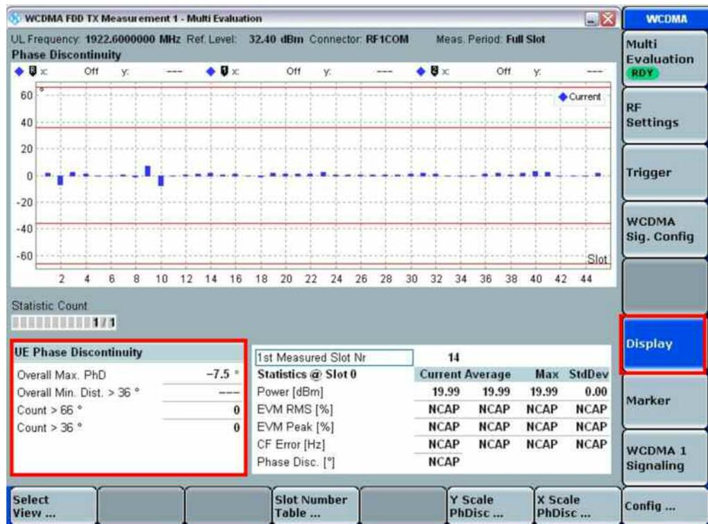
Fig. 32: Results from a phase discontinuity measurement.
