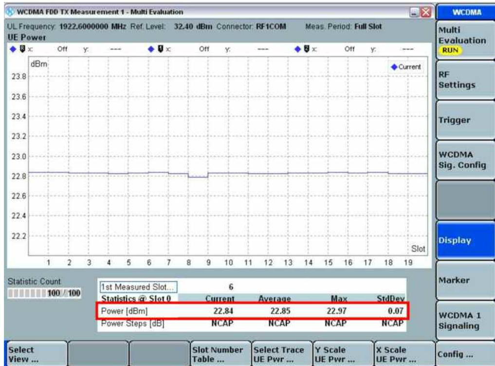
Fig. 9: Results from a maximum output power measurement.
