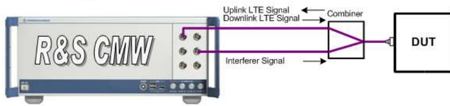
Test setup with interferer: two RF Frontends (Basic)
