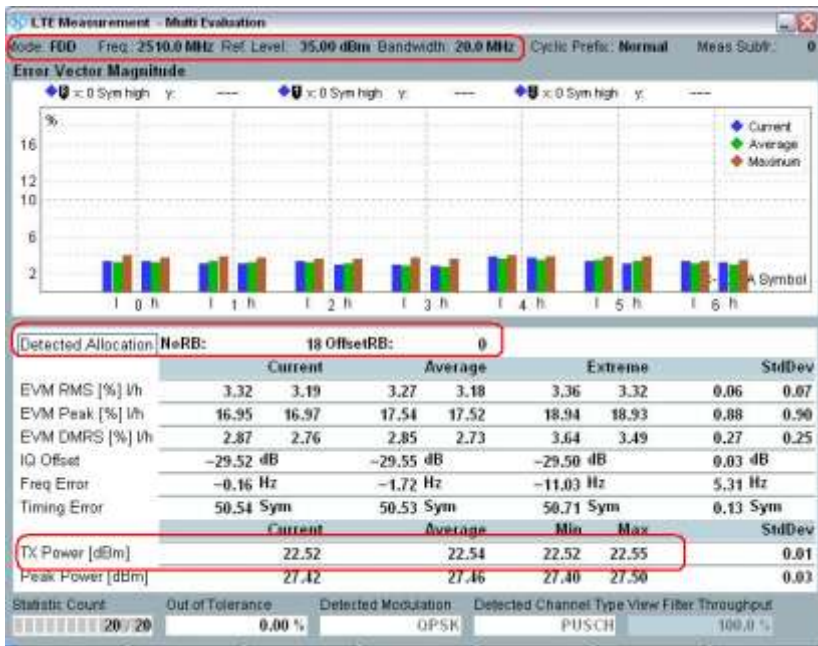
Fig. 15: Measurement results for UE maximum output power for 18 resource blocks.
