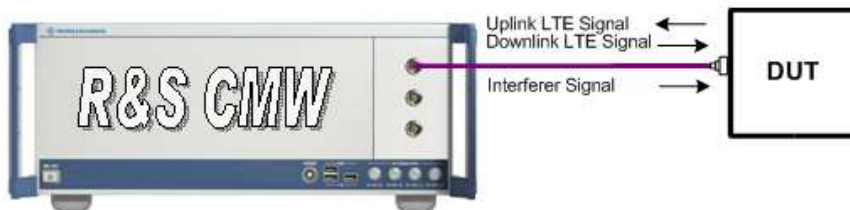
Test setup with interferer: one RF Frontend (Advanced)
