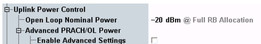
Fig. 12: Open Loop Nominal Power Settings
