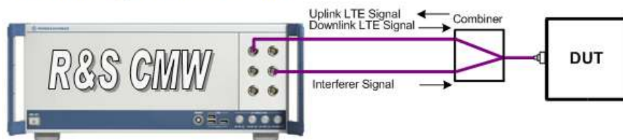
Test setup with interferer: two RF Frontends (Basic)
